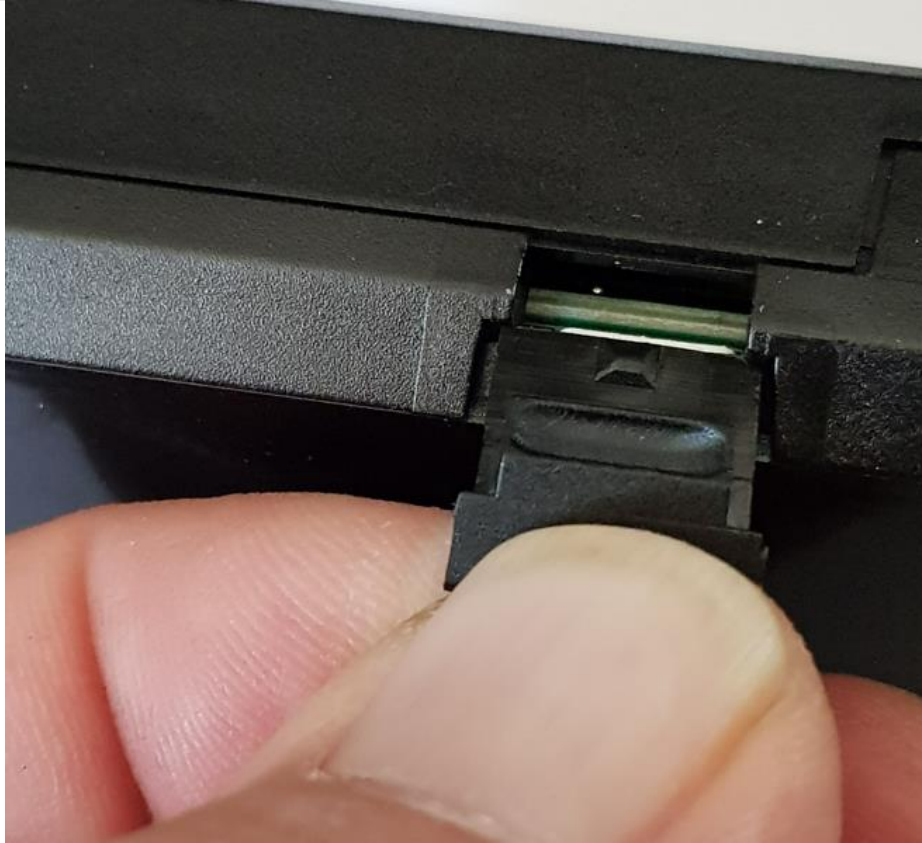
Figure 4: Close SIM cardholder door
