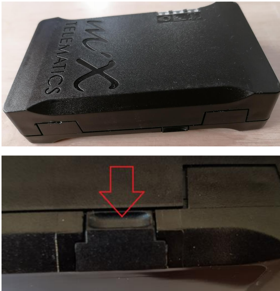
Figure 1: Open SIM card door
