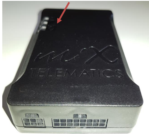
Figure 5 Unit orientated for GPS antenna to face towards the sky
