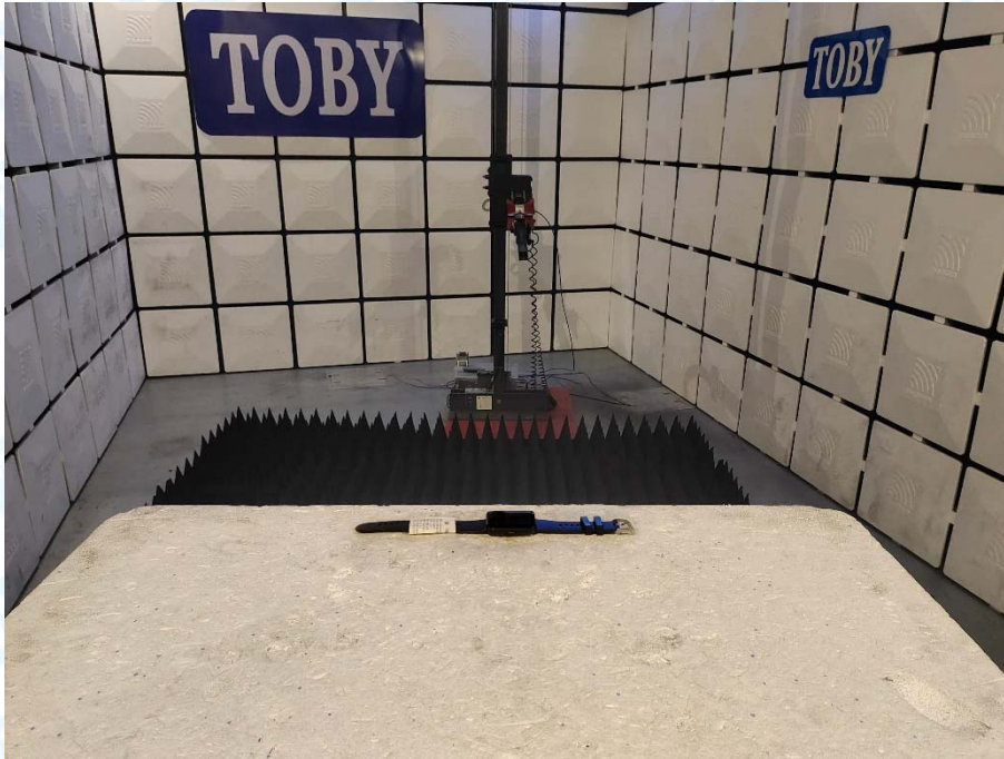
Photo of Setup for Conducted Emission
