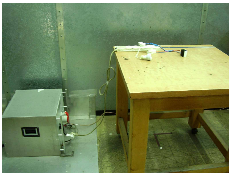
Photo 4. Conducted emission test setup
