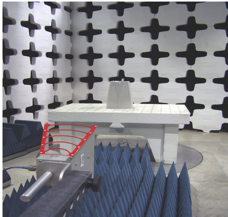
Photo 2. Radiated emission test setup
