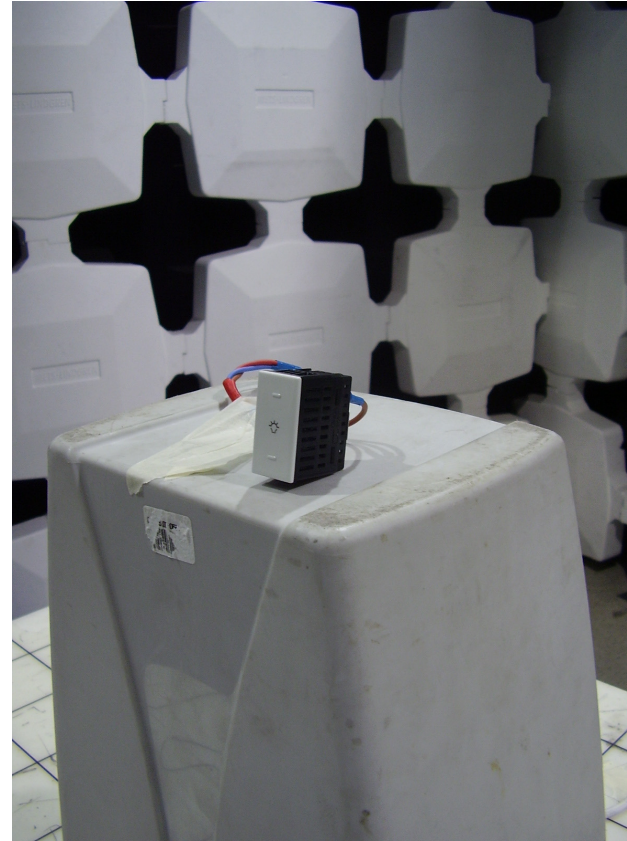
Photo 2. RE test setup
