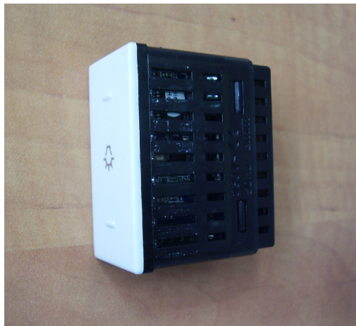
Photo 1. Smart switch side and rear view.
