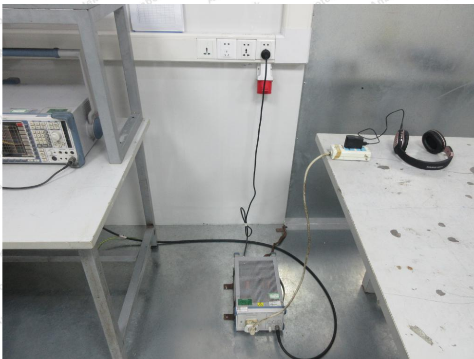
Photo of Conducted Emission Measurement
