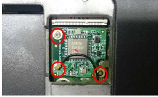
1. Unscrew 3 screws and remove the base cover
