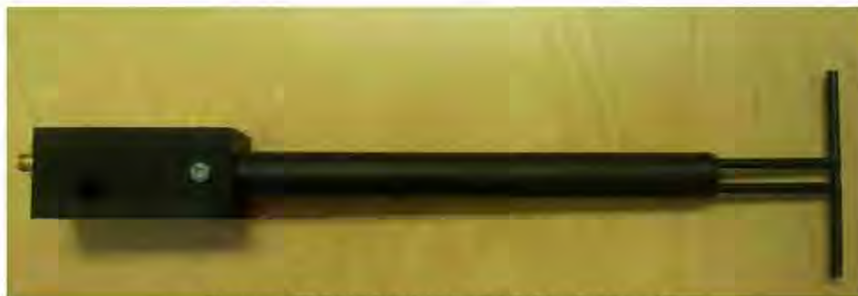
Figure 1 – MVG COMOSAR Validation Dipole
