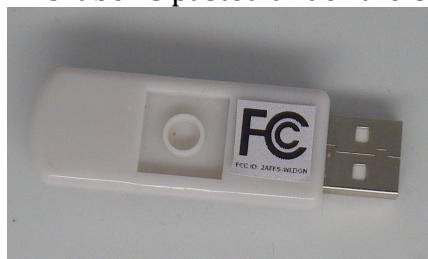
All labels are non-removable stickers. It is not etched in the injection mold because the same mold is used for different products.
