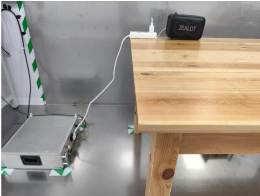
Conducted Emission at AC power line
