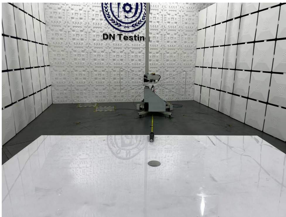
Radiated Emission Test View|(Below 1G)
