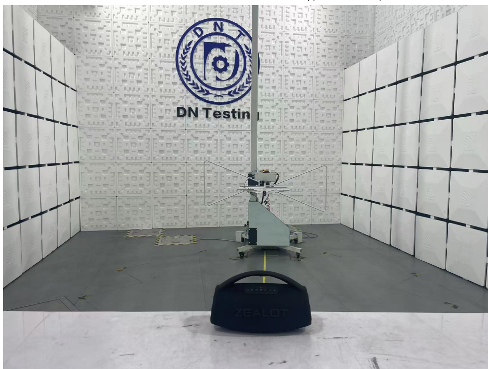
Radiated Emission Test View|(Below 1G)
