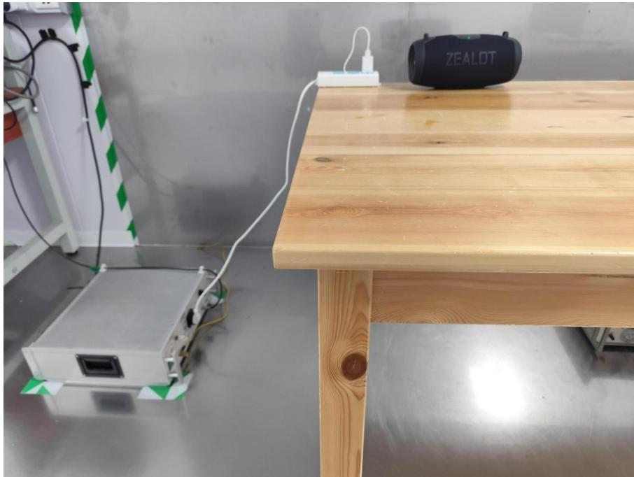
Conducted Emission at AC power line
