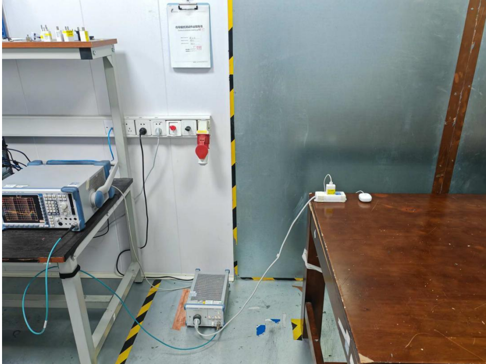
Conducted emissions at AC power line (150kHz-30MHz)
