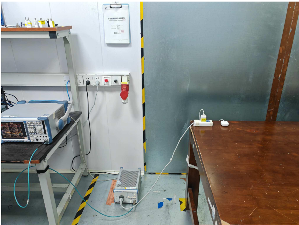
Conducted emissions at AC power line (150kHz-30MHz)
