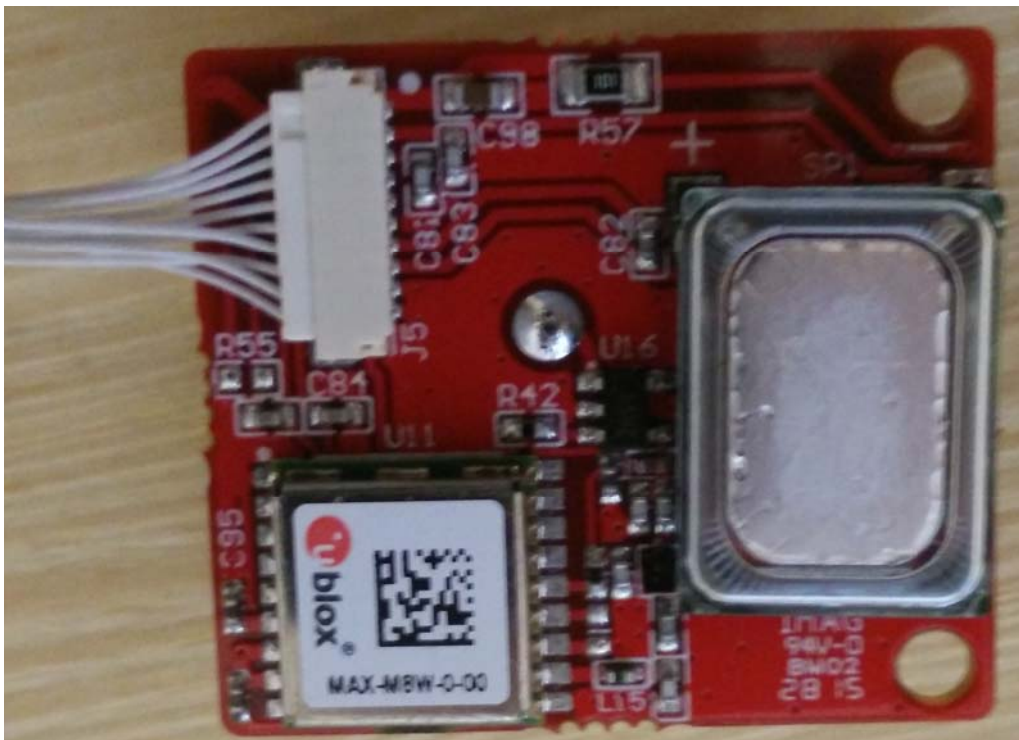
Figure 5 - Specifi-Kali Dog Tracking System - GPS PWB - Top
