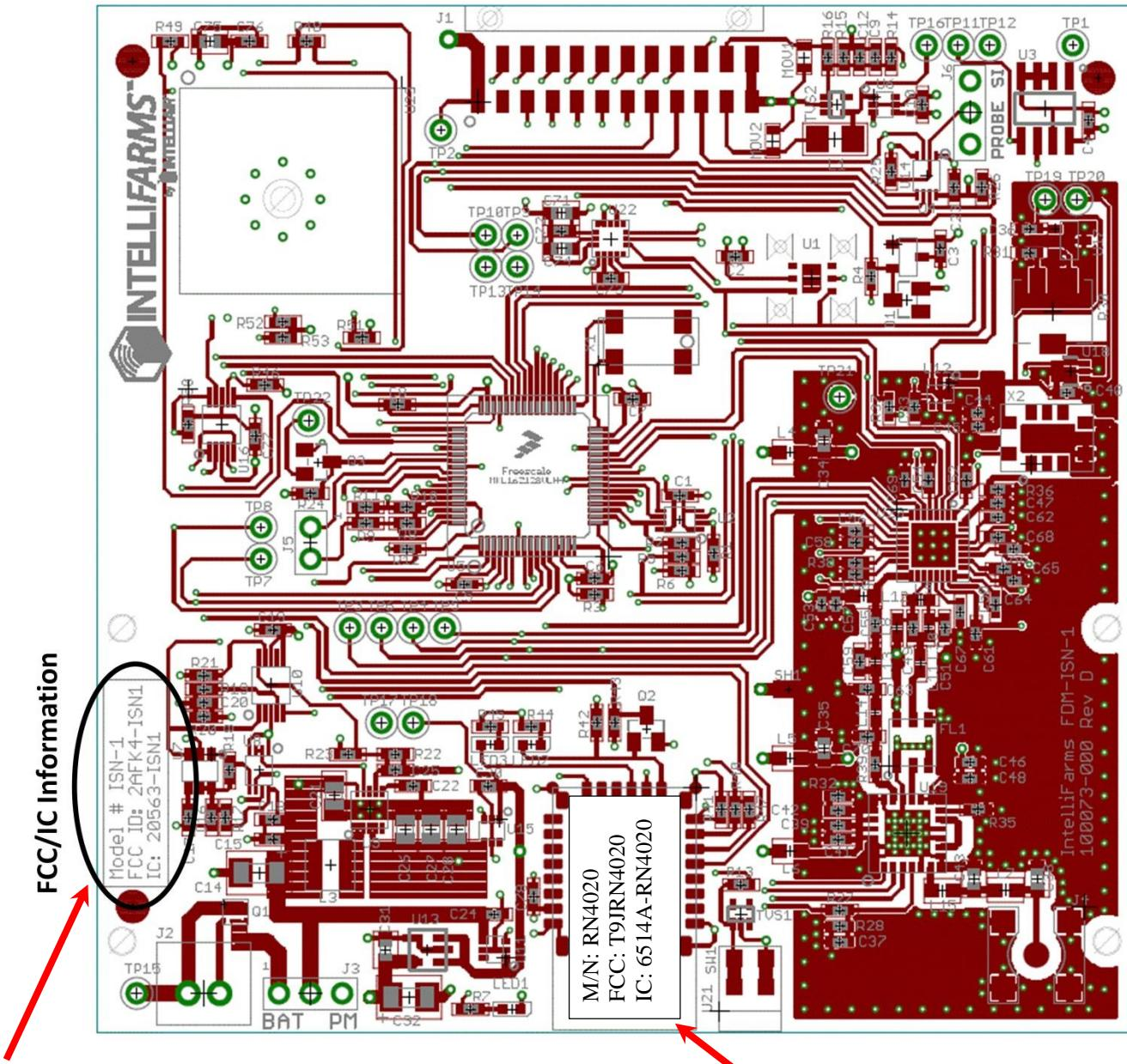
FCC and Industry Canada identifiers screened on PCB. RN4020 device and label.
