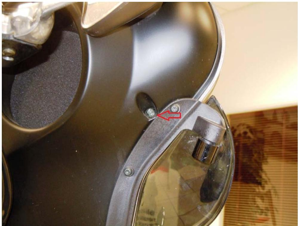
3. Locate and remove the two bolts at the bottom of the inner fairing one each side
