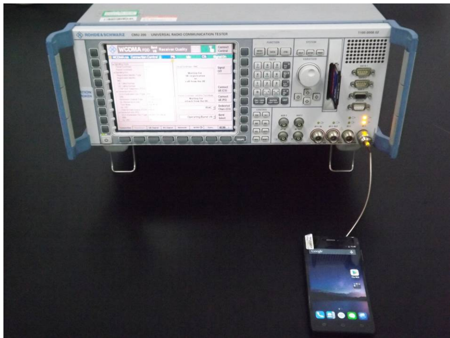
Photograph –2G&3G Conducted Test Setup
