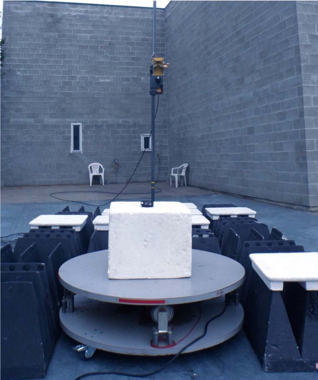
Figure E21.7 – Setup Photo – Radiated Measurements – 1GHz to 18 GHz, Horizontal
