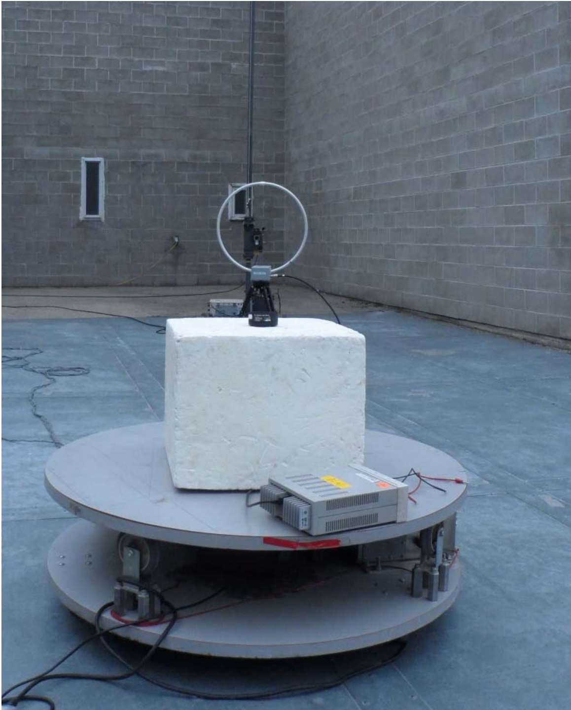
Figure E21.6 – Setup Photo – Radiated Measurements – 9kHz to 30MHz, Front Polarization
