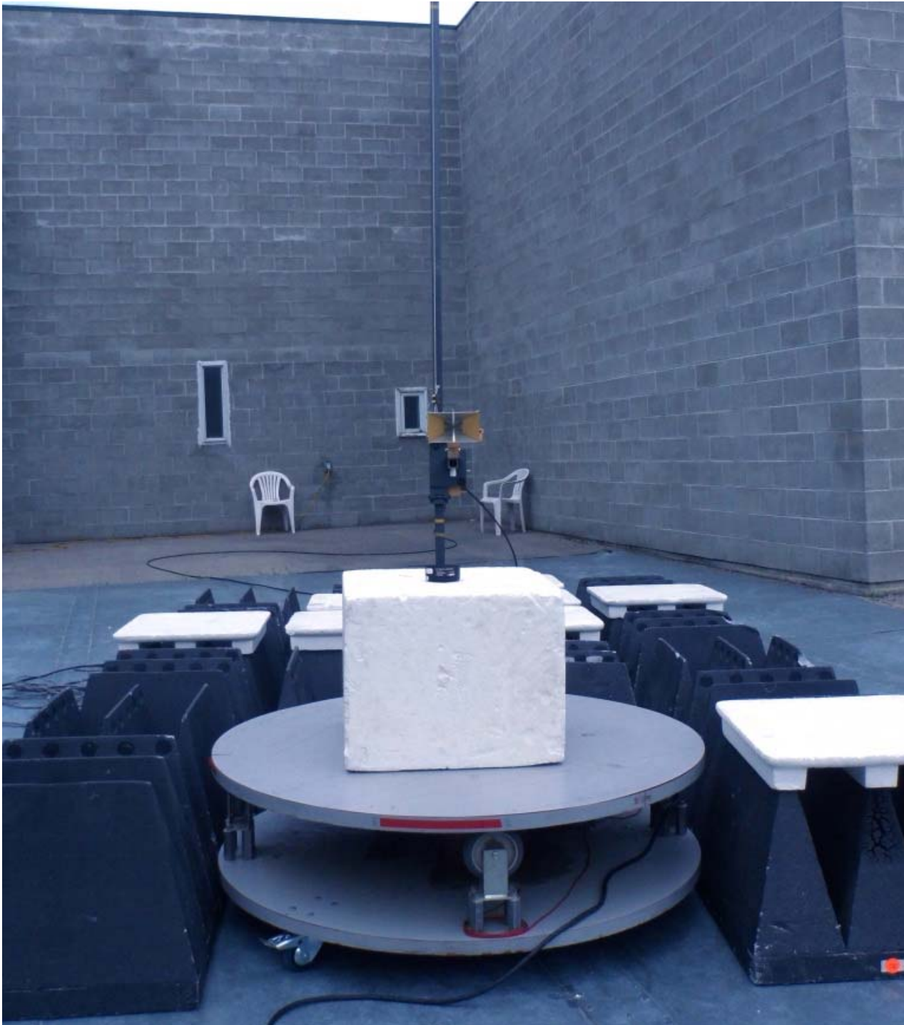
Figure E21.7 – Setup Photo – Radiated Measurements – 1GHz to 18 GHz, Vertical
