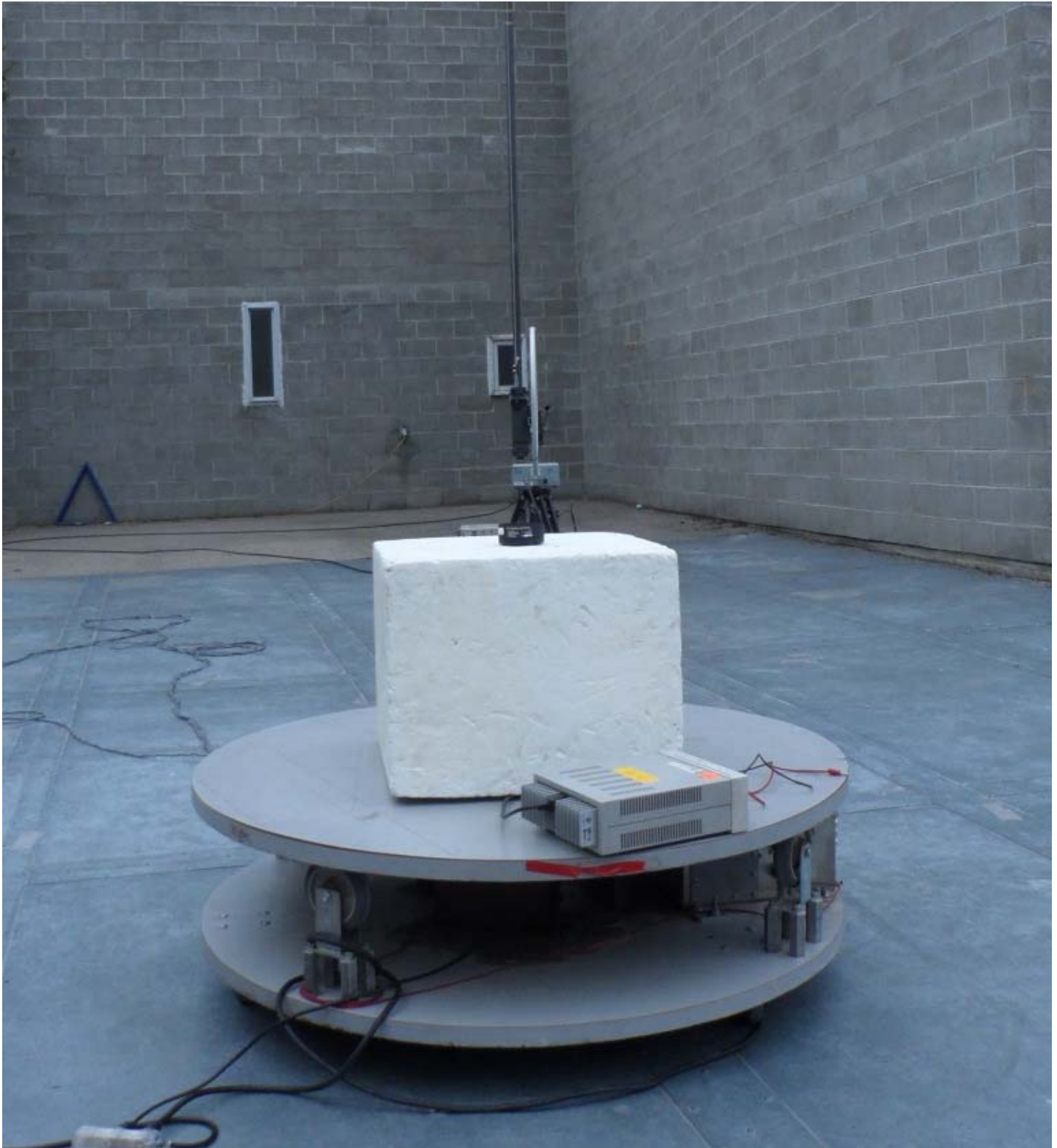
Figure E21.5 – Setup Photo – Radiated Measurements – 9kHz to 30MHz, Side Polarization
