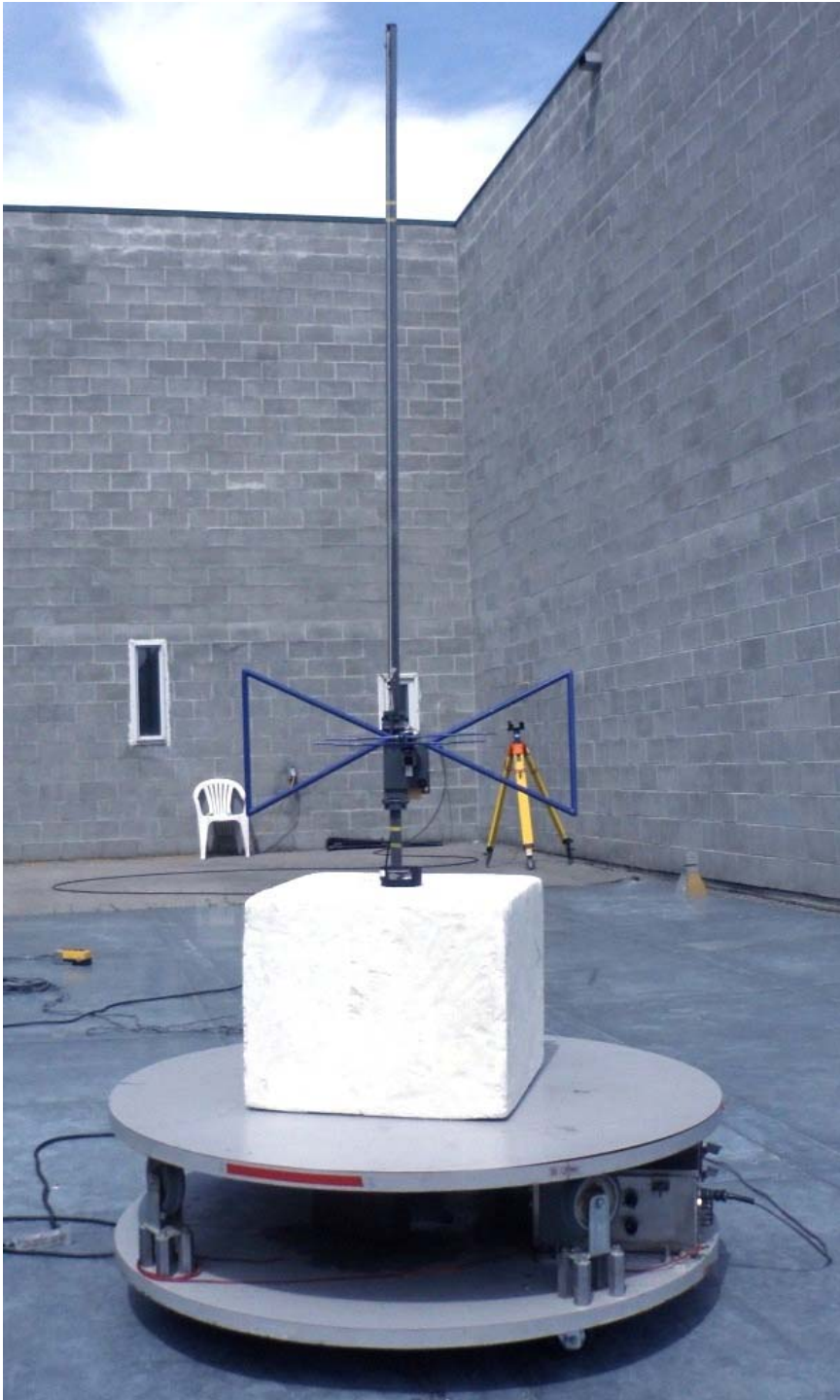
Figure E21.2 – Setup Photo – Radiated Measurements – 30MHz to 1000MHz, Horizontal
