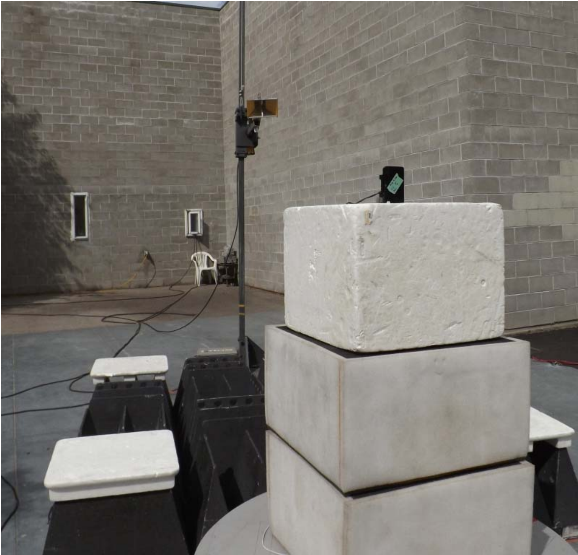
Figure E23.3 – Setup, Radiated Measurements 1 – 18GHz
