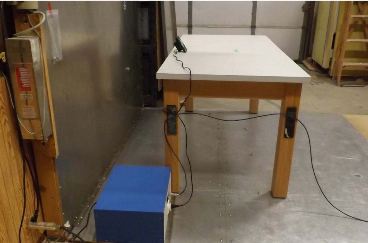
Figure E23.5 – Setup, Line Conducted Measurements
