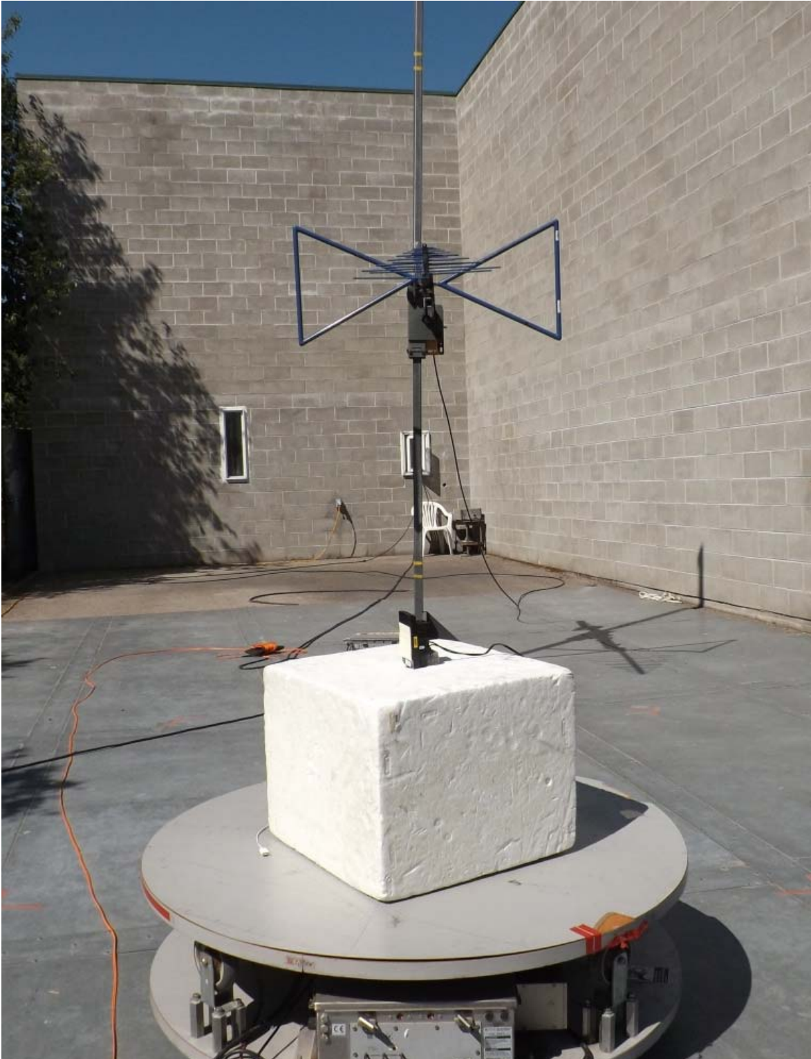
Figure E23.1 – Setup, Radiated Measurements Below 30MHz
