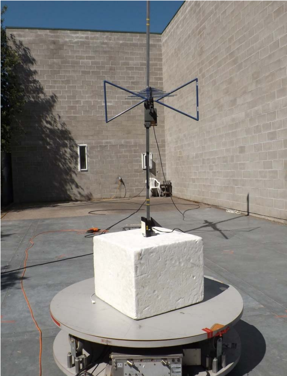
Figure E23.2 – Setup, Radiated Measurements 30 - 1000MHz
