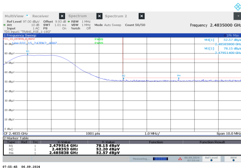
Figure 2.7.7-13: Radiated Band-Edge Emissions - 2 MBPS – Peak – 2480 MHz – Horizontal Polarization
