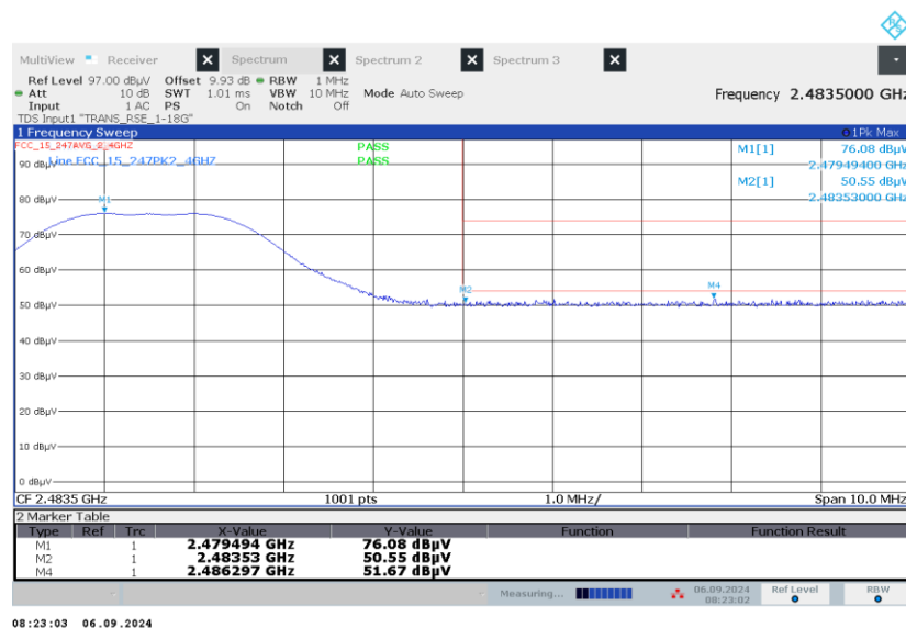
Figure 2.7.7-15: Radiated Band-Edge Emissions - 2 MBPS – Peak – 2480 MHz – Vertical Polarization
