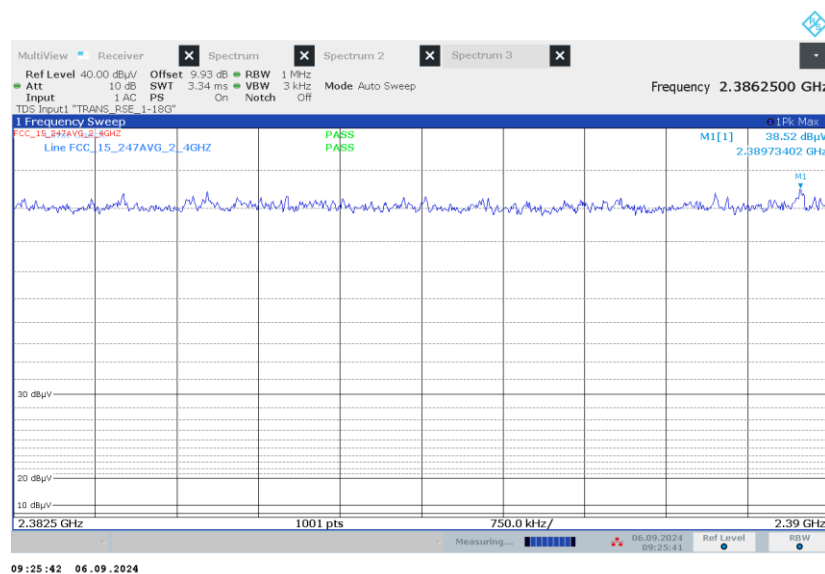
Figure 2.7.7-4: Radiated Band-Edge Emissions - 1 MBPS – Average – 2402 MHz – Vertical Polarization
