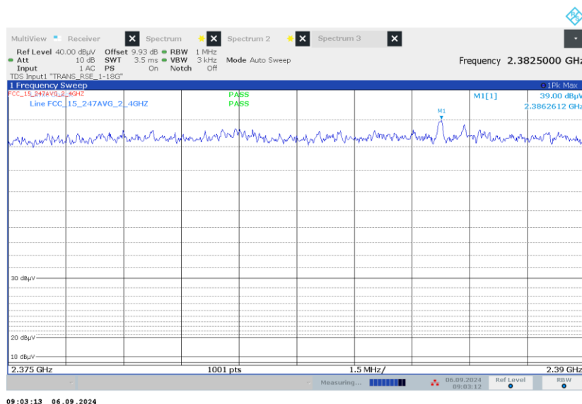
Figure 2.7.7-2: Radiated Band-Edge Emissions - 1 MBPS – Average – 2402 MHz – Horizontal Polarization
