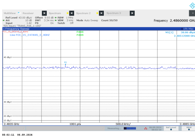
Figure 2.7.7-14: Radiated Band-Edge Emissions - 2 MBPS – Average – 2480 MHz – Horizontal Polarization
