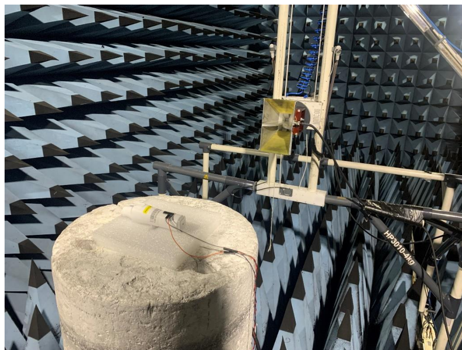
Figure 10 – Test Setup Photo BLE (Radiated), Z-Orientation, 0 Degrees
