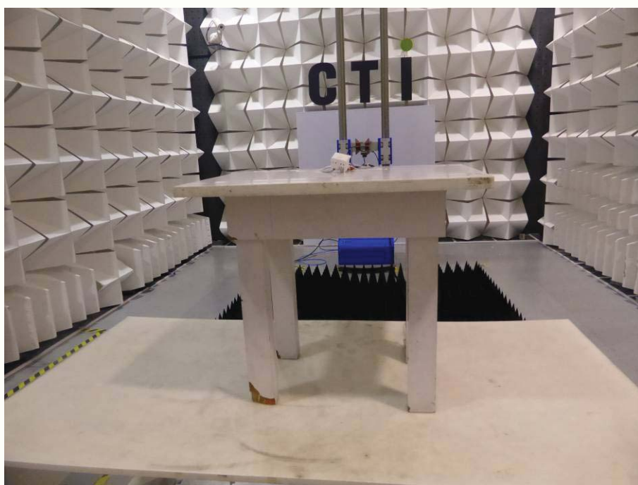
Radiated spurious emission Test Setup-2(Above 1GHz)
