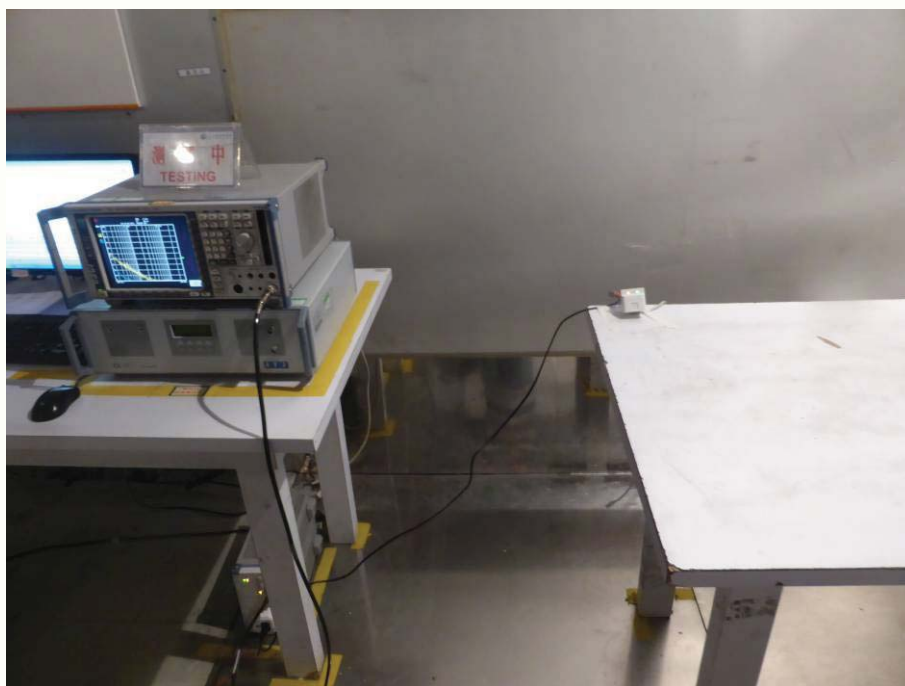
Conducted spurious emission Test Setup
