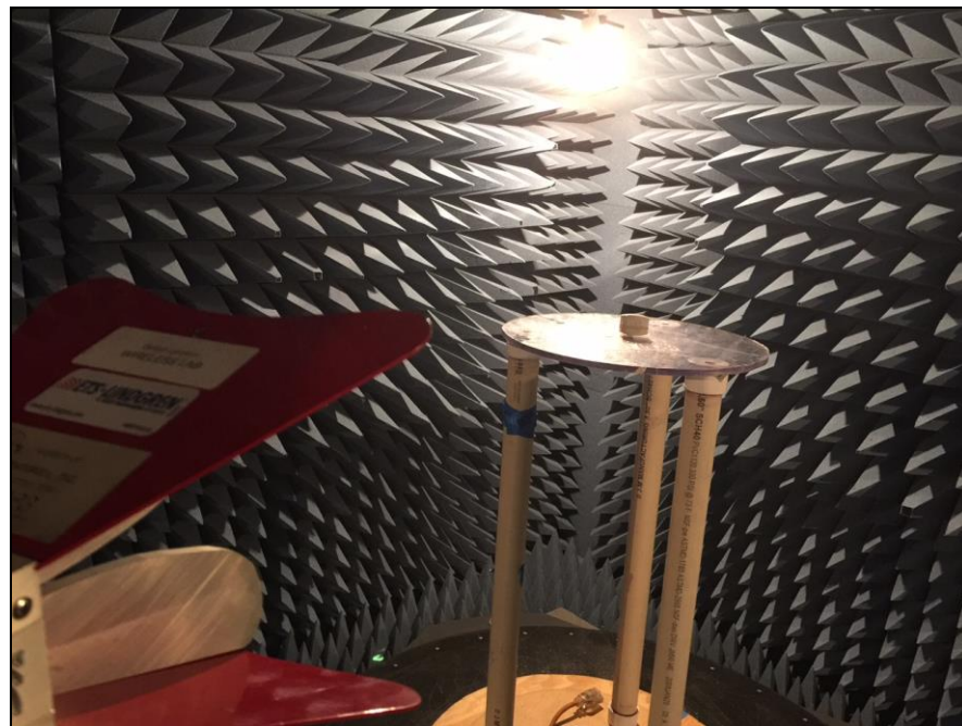
Photograph 2. Radiated Spurious Emissions, Test Setup, Above 1 GHz
