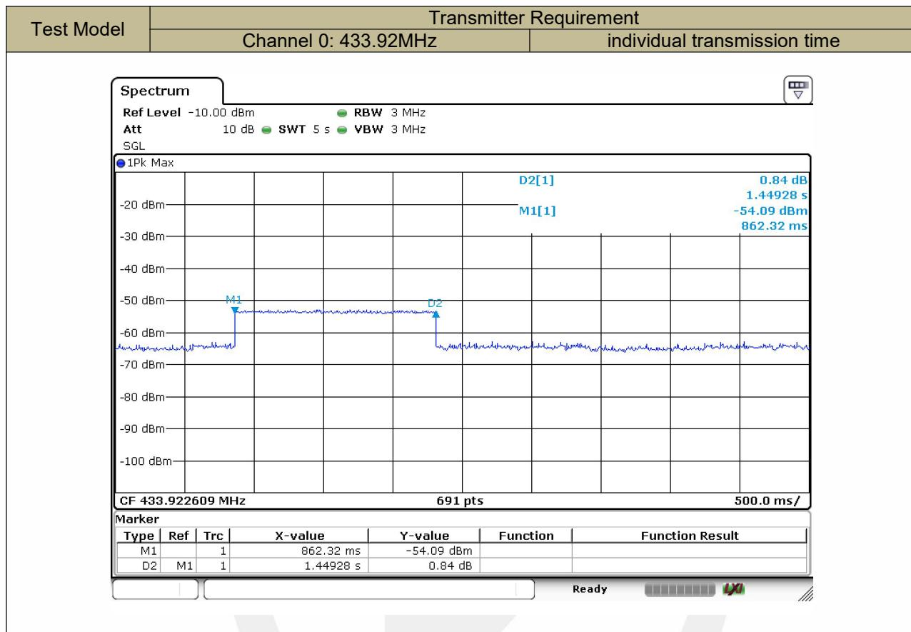
The transmitters deactivated within 1.5 seconds of the button being released and no transmissions were detected within 5 seconds of release.
