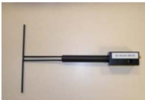
Figure 1 – Satimo COMOSAR Validation Dipole
