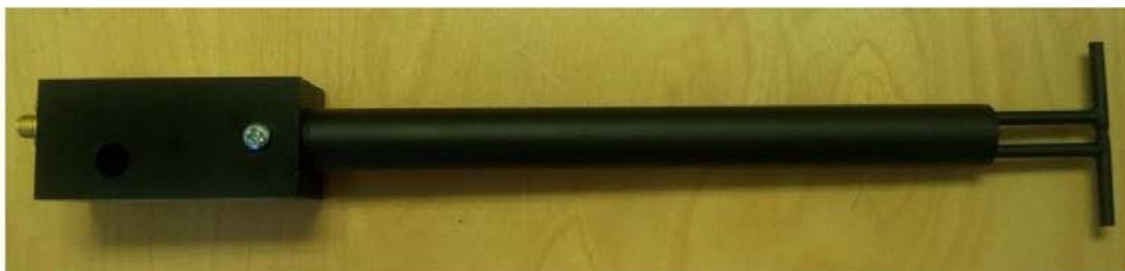
Figure 1 – MVG COMOSAR Validation Dipole
