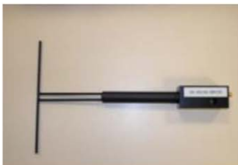
Figure 1 – Satimo COMOSAR Validation Dipole
