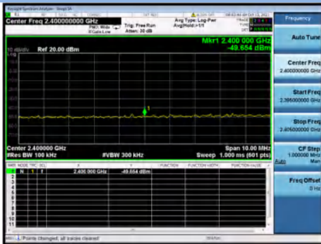
802.11g CHANNEL 3, Carrier level
