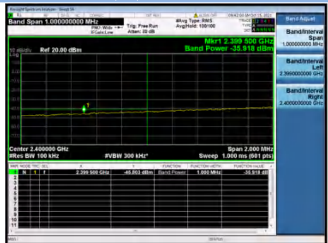
802.11ax-20 MHz(SU) CHANNEL 1, Reference level
