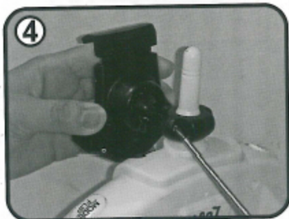
4. Use the screwdriver to tighten the bolt up.
