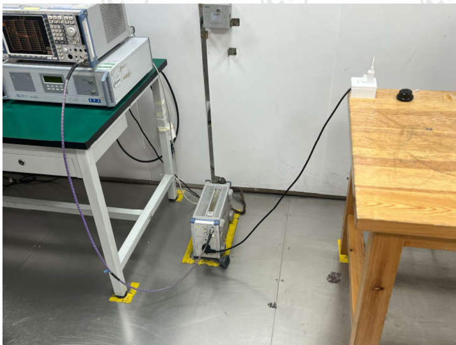
Conducted Emissions Test Setup
