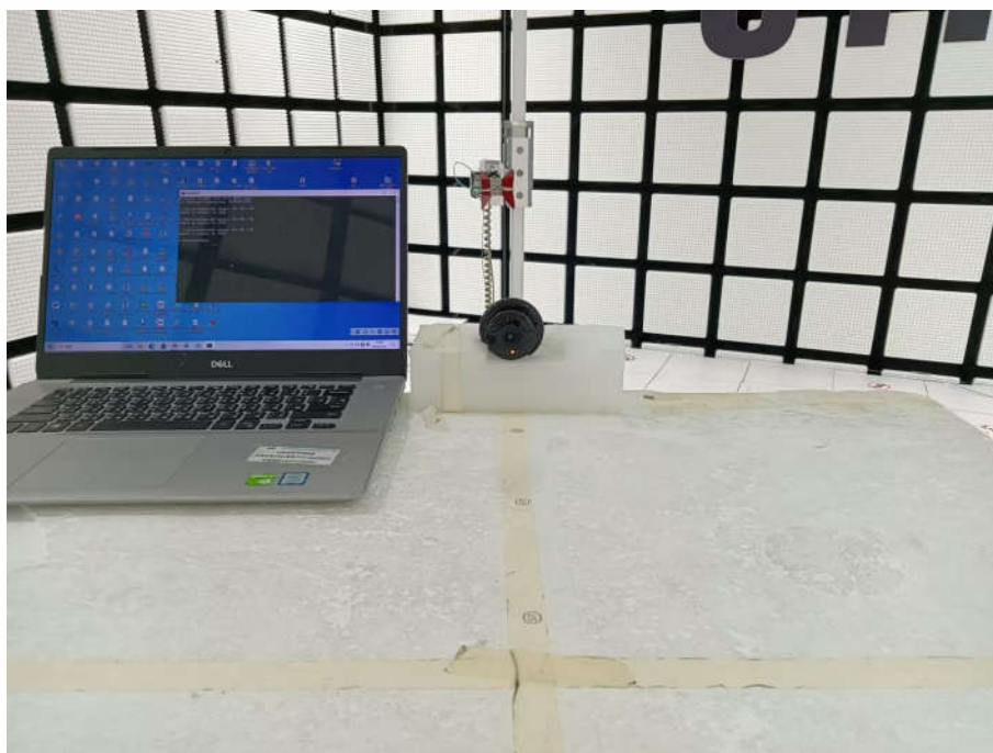
Radiated spurious emission Test Setup-2(Above 1GHz)
