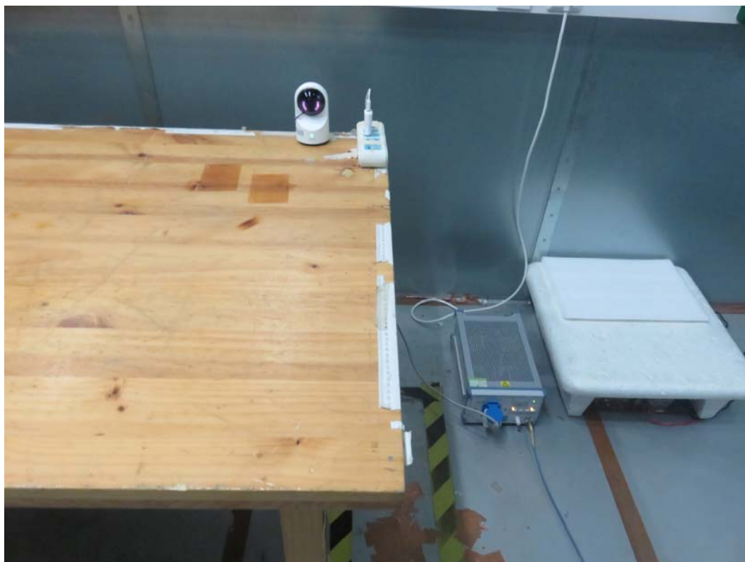
Picture 3 Conducted Emission Test Setup
