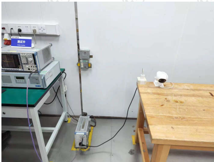
Conducted Emissions Test Setup
