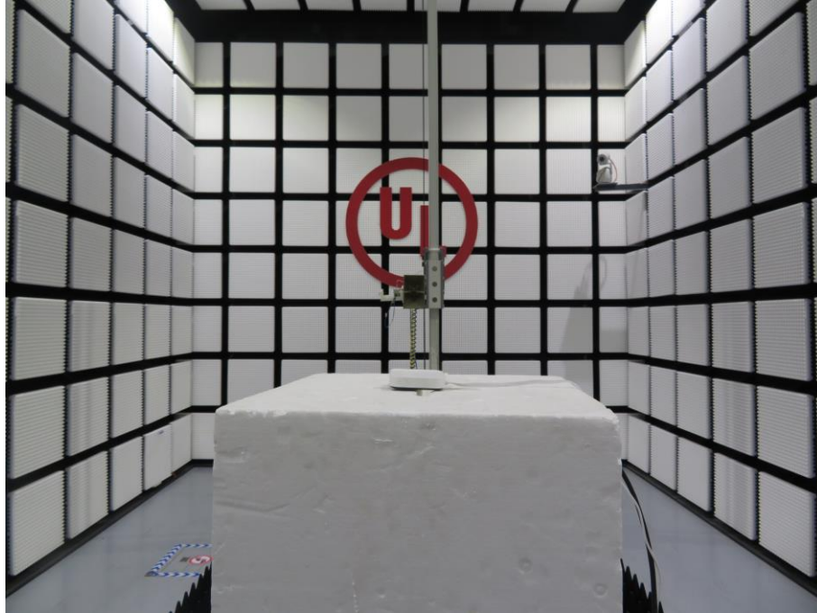
RADIATED RF MEASUREMENT SETUP (ABOVE 1 GHz)
