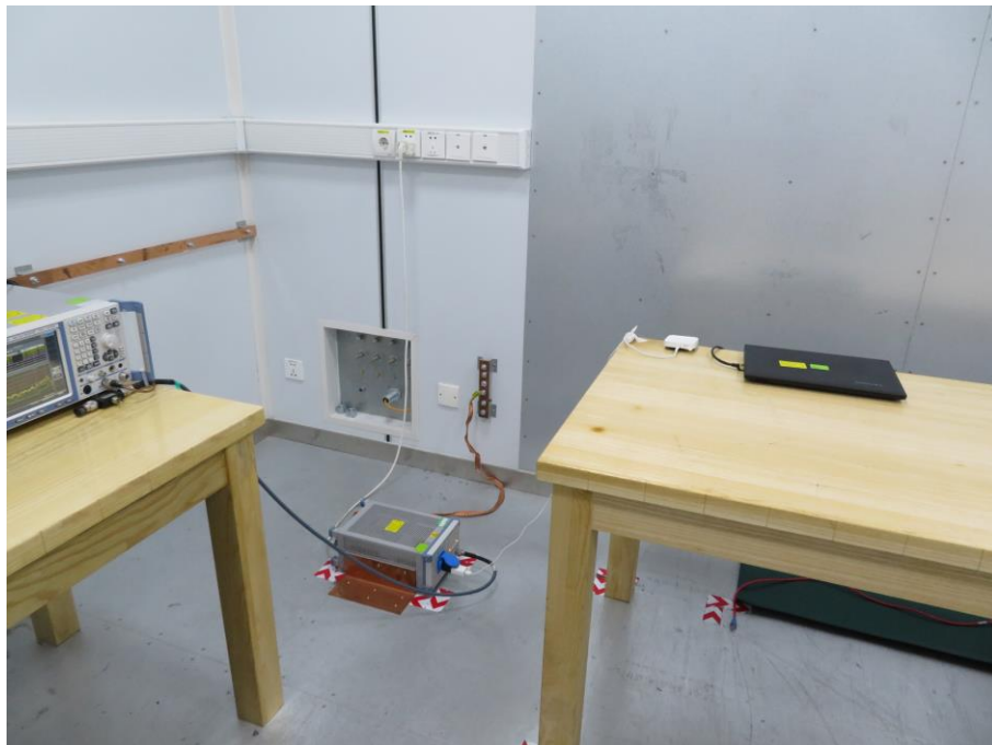
POWERLINE CONDUCTED EMISSIONS MEASUREMENT SETUP
