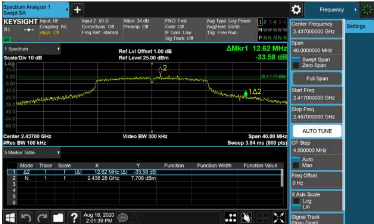
Figure 5: 6dB Bandwidth and 99% Bandwidth, 802.11g, 2437MHz
