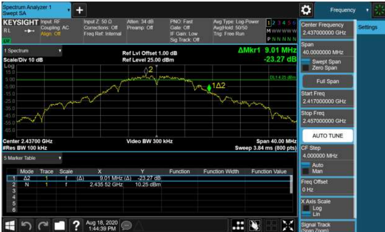
Figure 2: 6dB Bandwidth and 99% Bandwidth, 802.11b, 2437MHz
