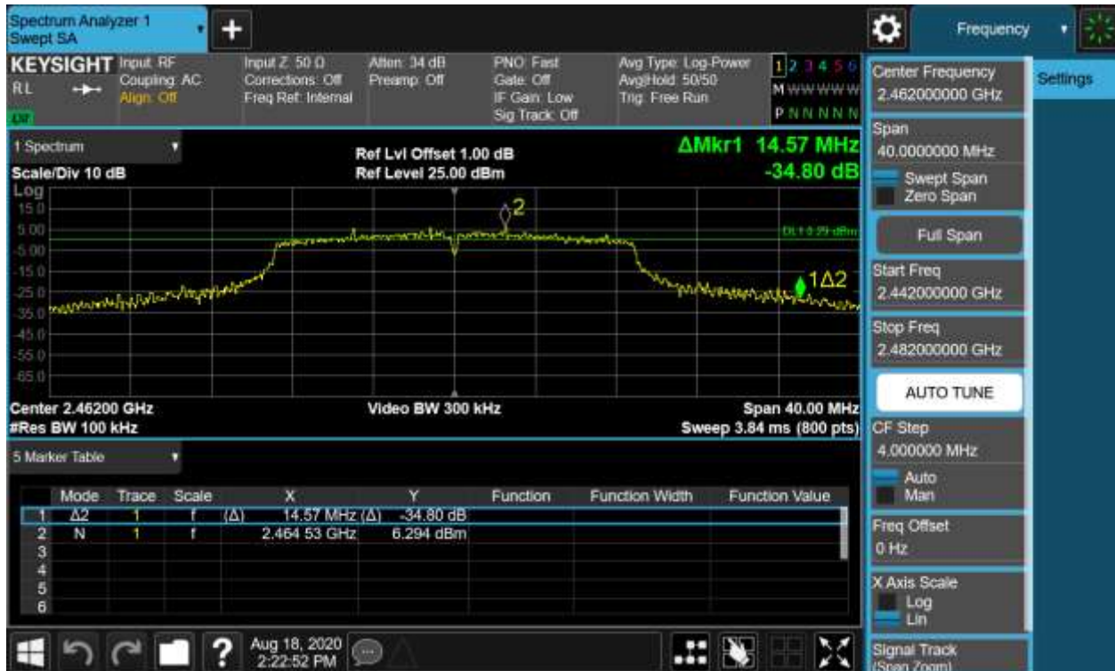
Figure 9: 6dB Bandwidth and 99% Bandwidth, 802.11n(HT20), 2462MHz
