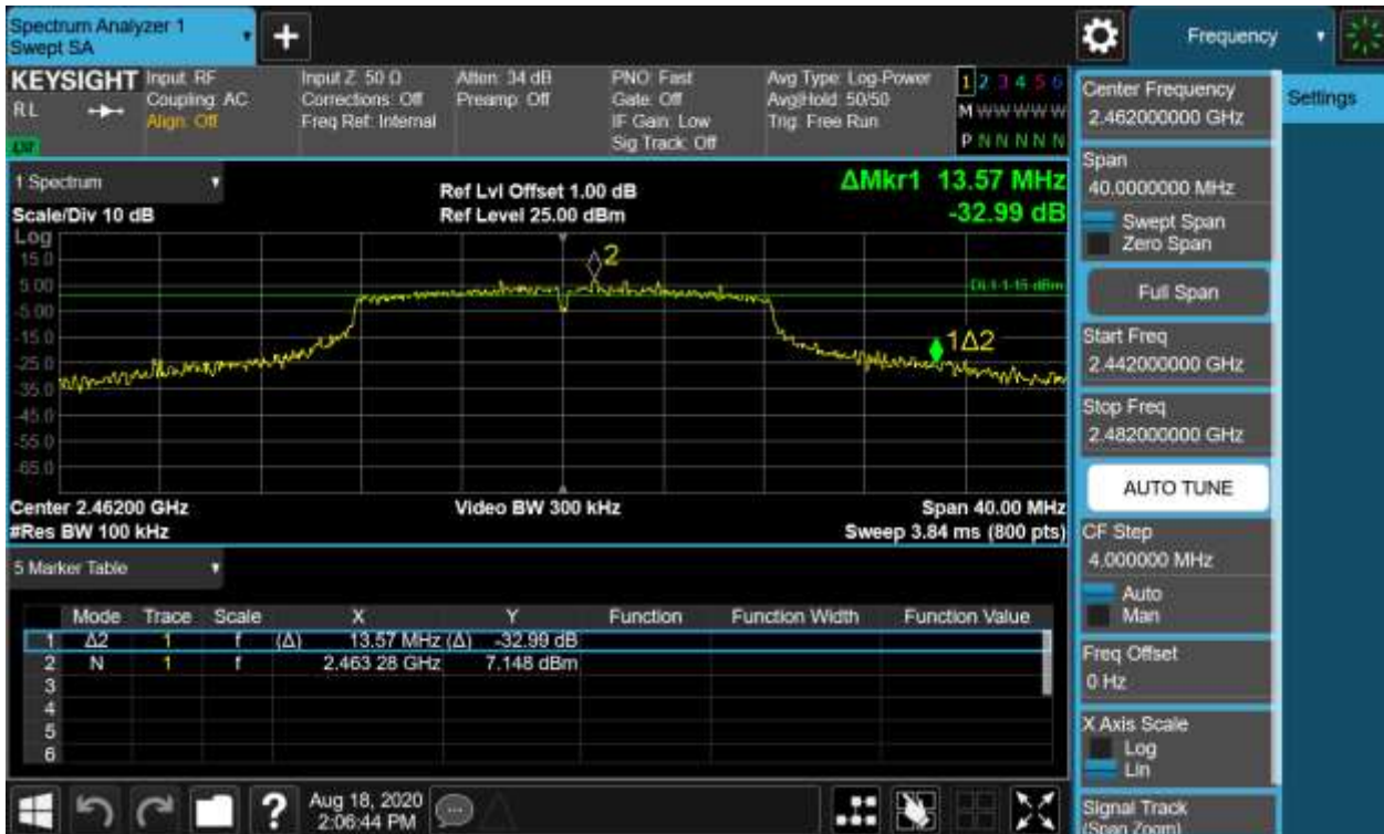
Figure 6: 6dB Bandwidth and 99% Bandwidth, 802.11g, 2462MHz
