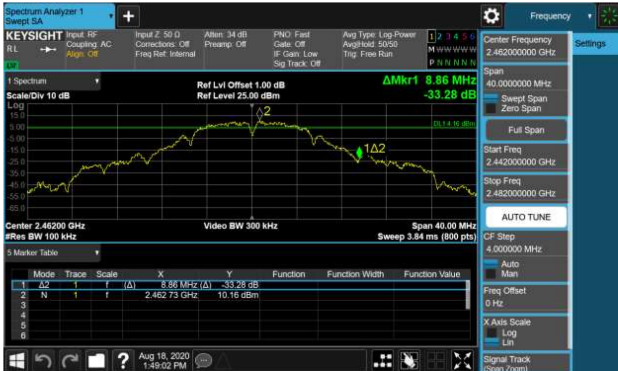
Figure 3: 6dB Bandwidth and 99% Bandwidth, 802.11b, 2462MHz
