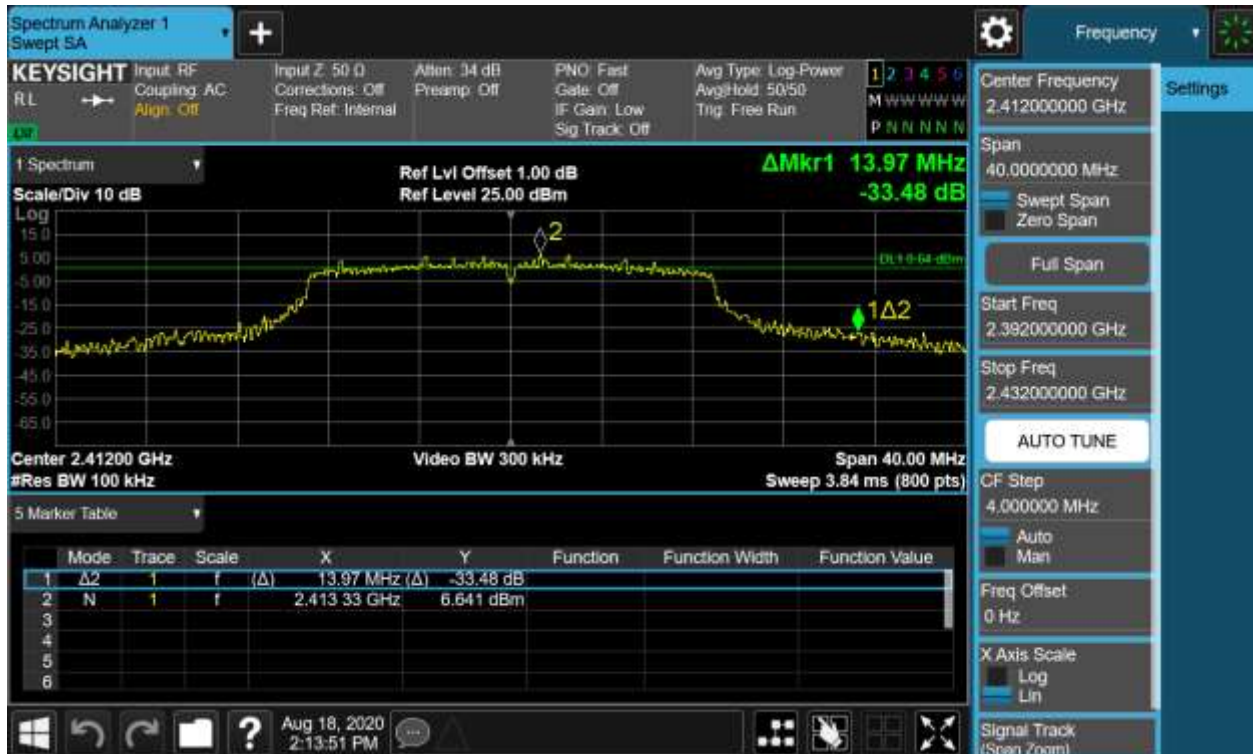
Figure 7: 6dB Bandwidth and 99% Bandwidth, 802.11n(HT20), 2412MHz
