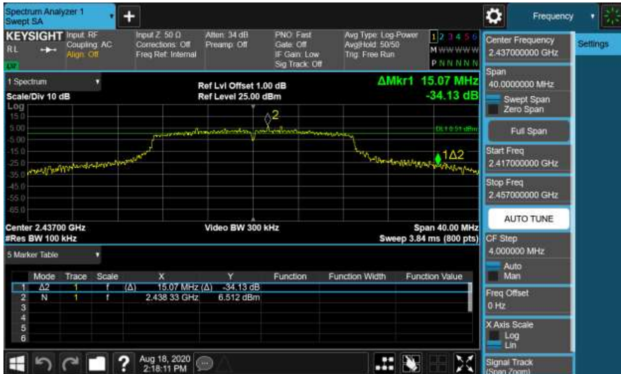
Figure 8: 6dB Bandwidth and 99% Bandwidth, 802.11n(HT20), 2437MHz
