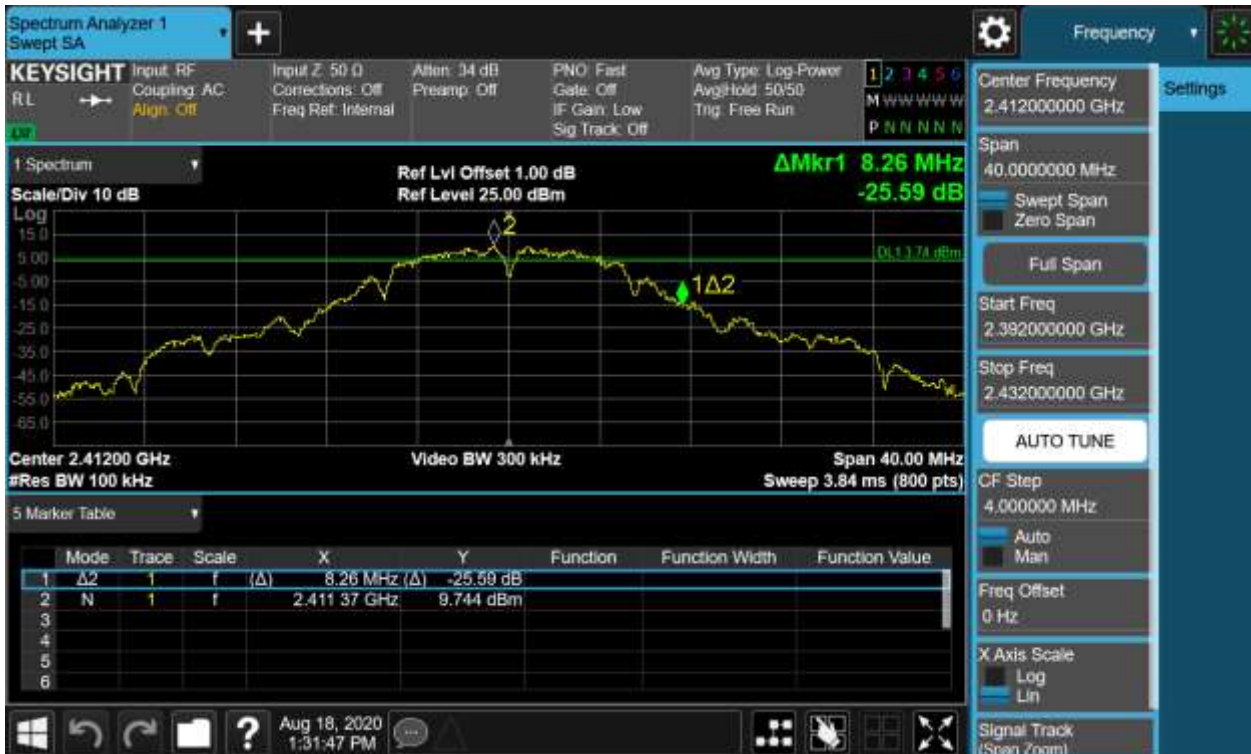
Figure 1: 6dB Bandwidth and 99% Bandwidth, 802.11b, 2412MHz
