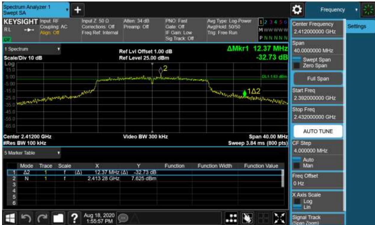
Figure 4: 6dB Bandwidth and 99% Bandwidth, 802.11g, 2412MHz
