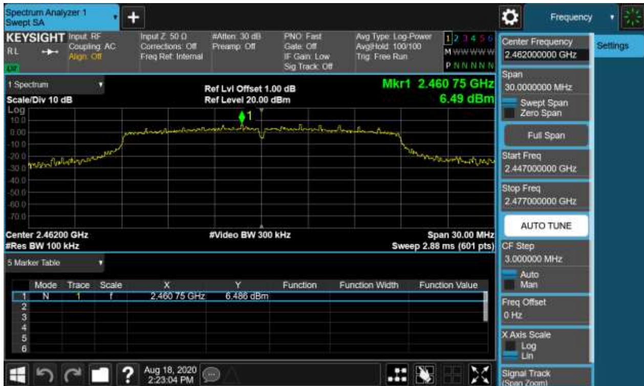
Figure 27: Conducted Spurious Emission & Authorized-band band-edge, 802.11n(HT20), 2462MHz Carrier Level
