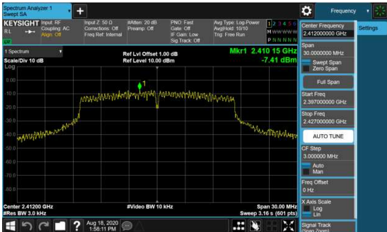
Figure 13: Power Spectral Density, 802.11g, 2412MHz
