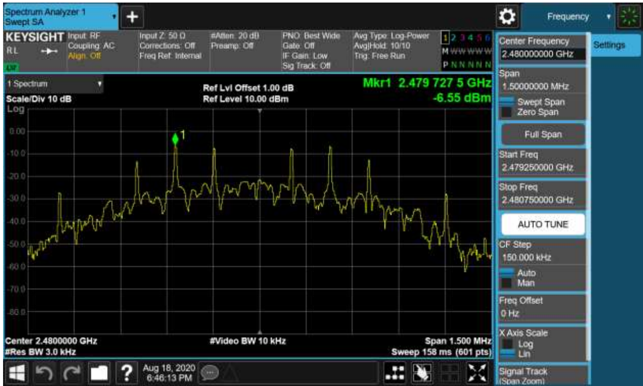
Figure 9: Power Spectral Density, 2480MHz
