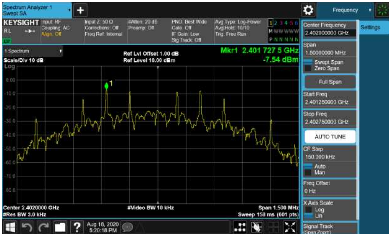
Figure 7: Power Spectral Density, 2402MHz
