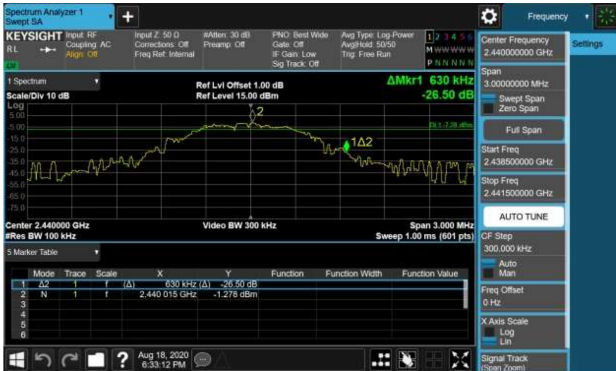
Figure 5: 6dB Bandwidth and 99% Bandwidth, 2440MHz
