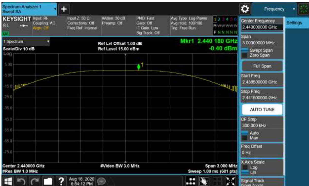
Figure 2: Peak Output Power, 2440MHz
