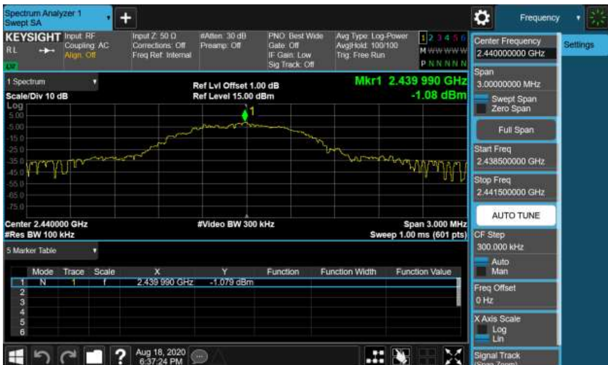
Figure 11: Conducted Spurious Emission & Authorized-band band-edge, 2440MHz, BLE Carrier Level
