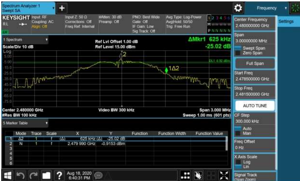
Figure 6: 6dB Bandwidth and 99% Bandwidth, 2480MHz
