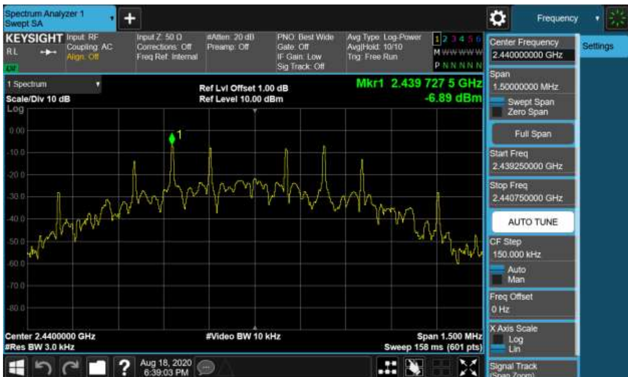
Figure 8: Power Spectral Density, 2440MHz
