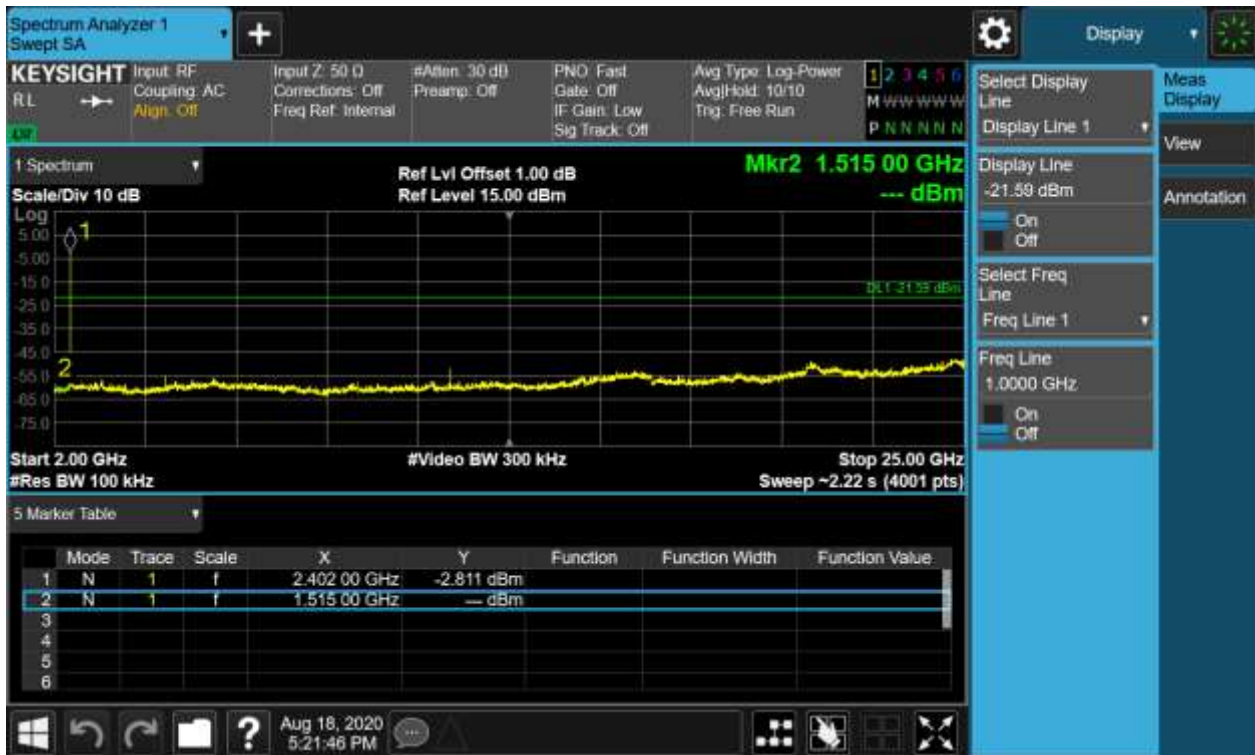
Figure 11: Conducted Spurious Emission & Authorized-band band-edge, 2440MHz, BLE Carrier Level
