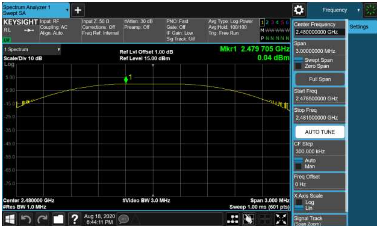
Figure 3: Peak Output Power, 2480MHz
