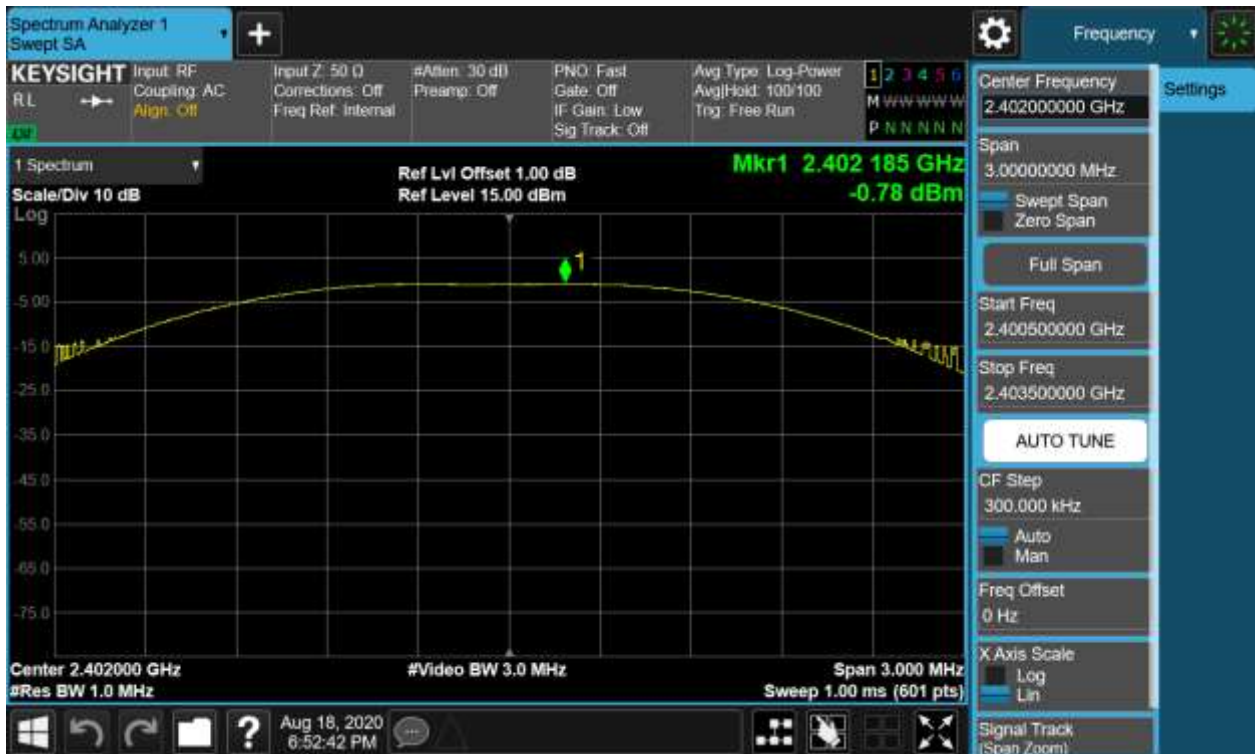
Figure 1: Peak Output Power, 2402MHz
