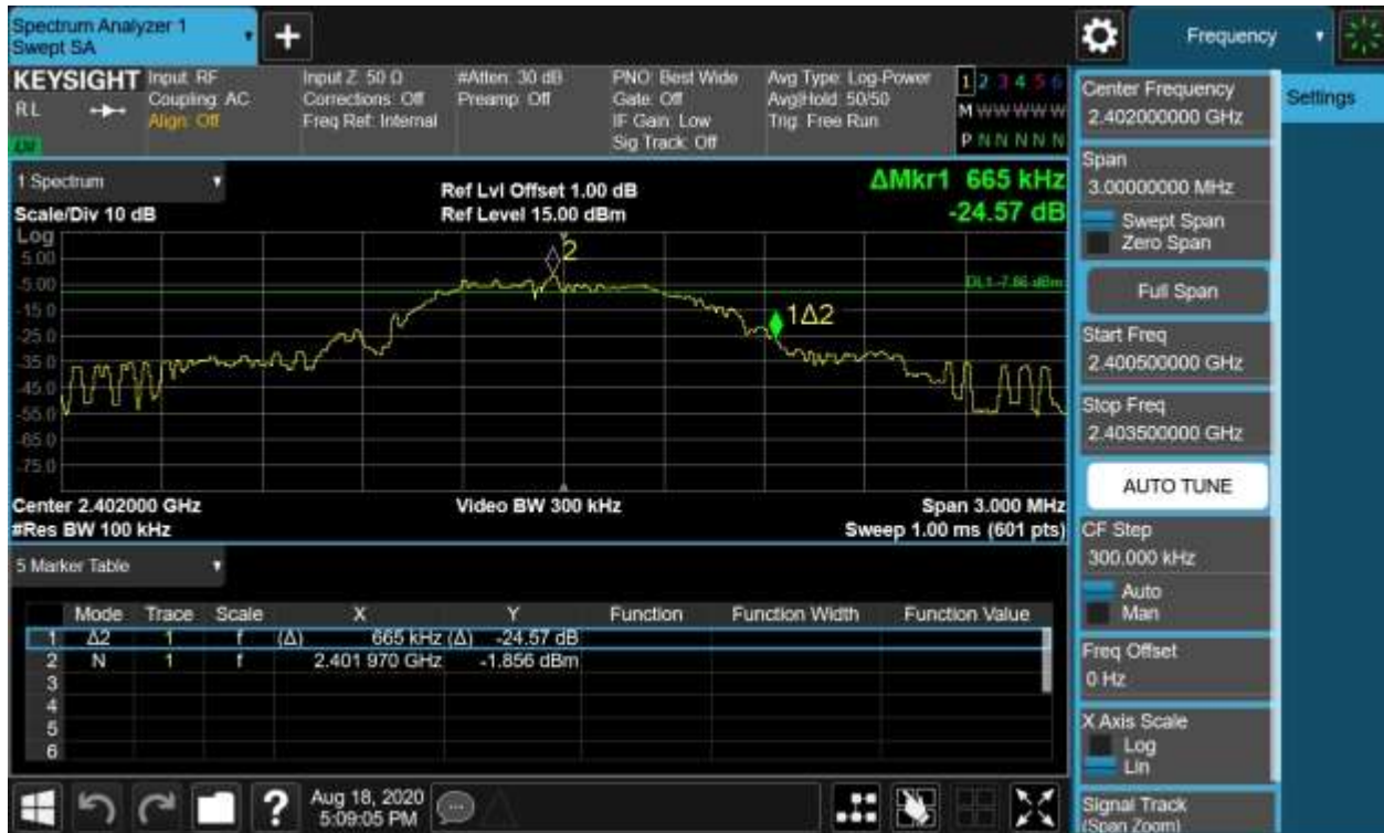
Figure 4: 6dB Bandwidth and 99% Bandwidth, 2402MHz
