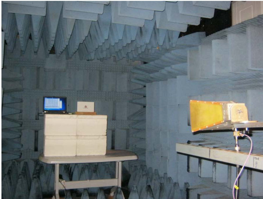
Figure 6. Radiated Emission Test, 1000-18,000MHz band
