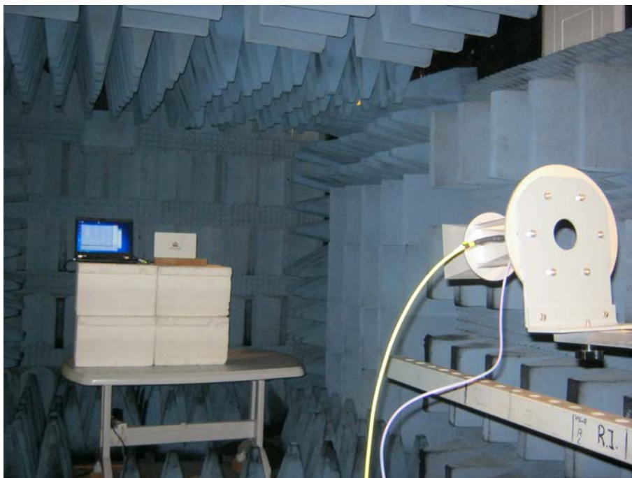
Figure 7. Radiated Emission Test, 18,000-26,500MHz band
