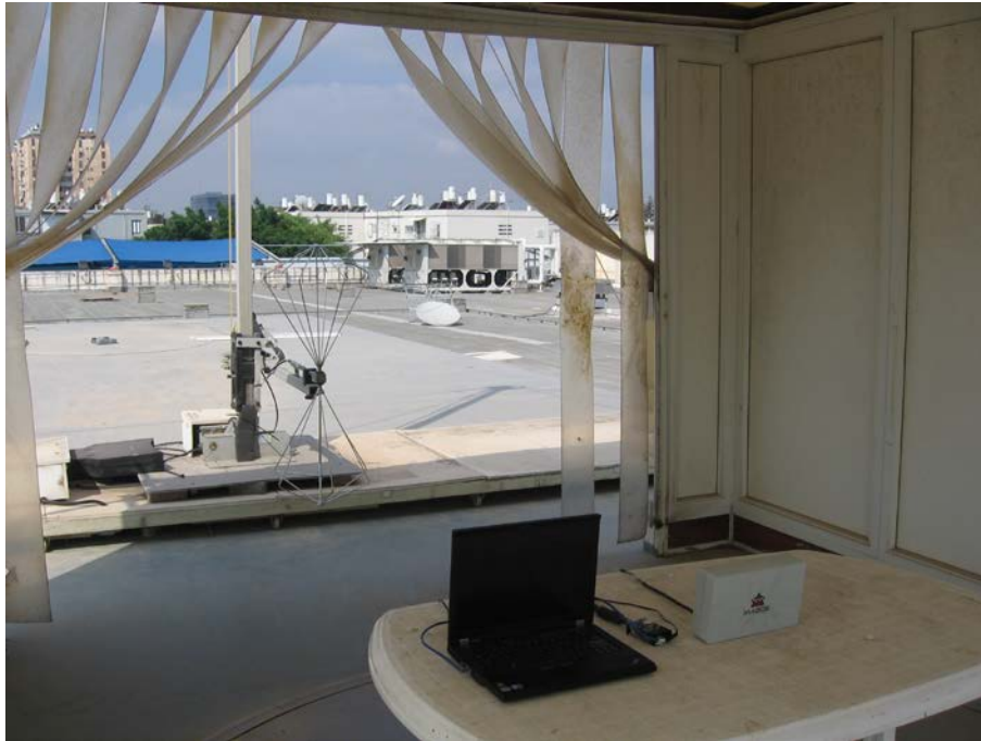
Figure 4. Radiated Emission Test, 30-200MHz band
