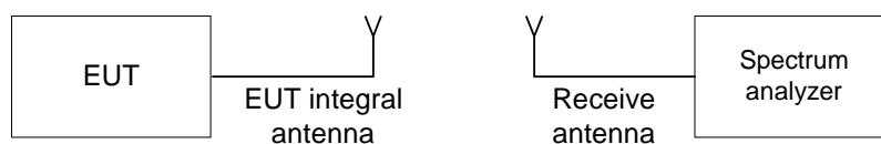
Figure 7.3.1 Occupied bandwidth test setup
