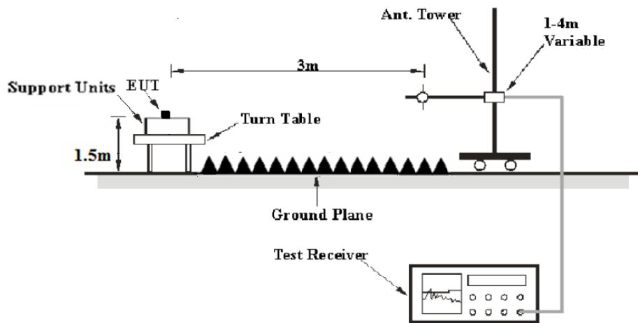
The radiated emission tests were performed in the 3 meters test site, using the setup accordance with the ANSI C63.10 - 2013. The specification used was the FCC § 15.209, 15.205 and 15.231.
