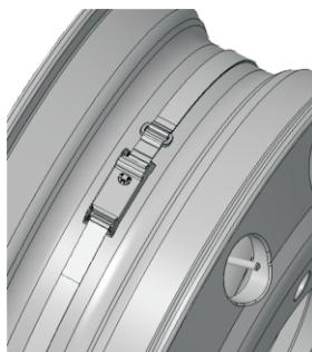
Place the sensor on bottom of wheel, ensuring arrow direction the same side of valve.
