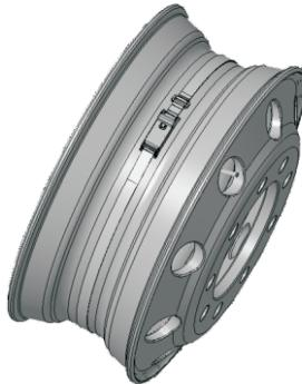
Fasten sensor with strap by hand, make sure the sensor stuck on wheel.
