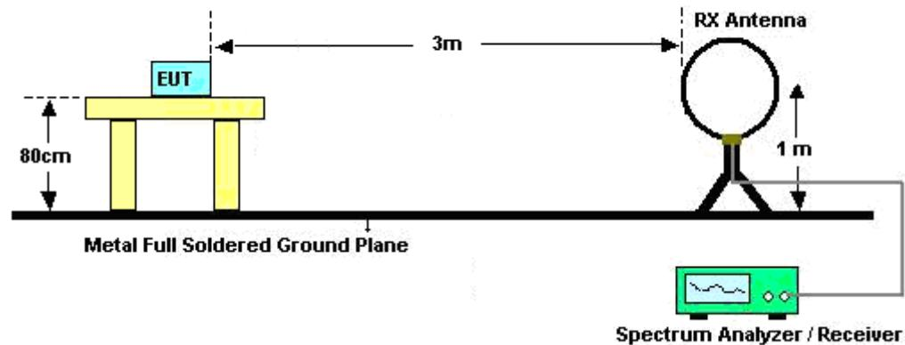
For radiated emissions from 30MHz to 1GHz
