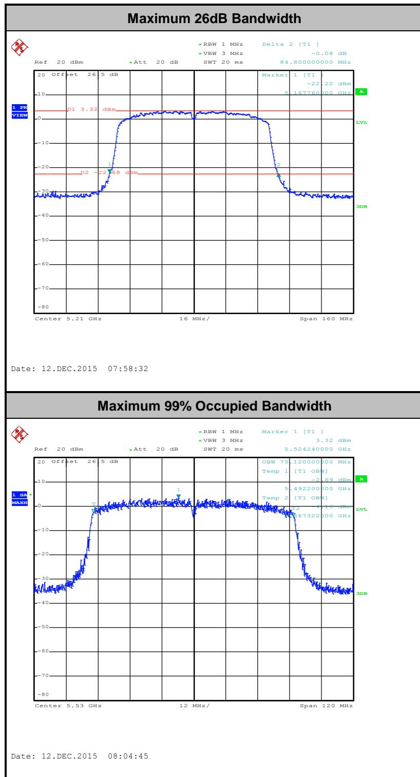
Note : The occupied channel bandwidth is maintained within the band of operation for all of the modulations.
