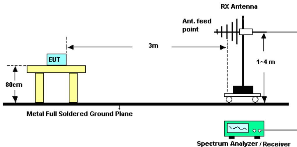
**For radiated emissions above 1GHz**
