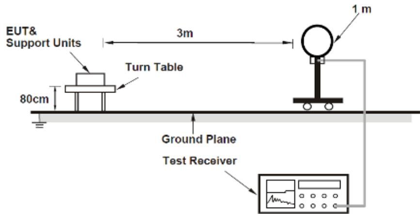
For Radiated emission 30MHz to 1GHz
