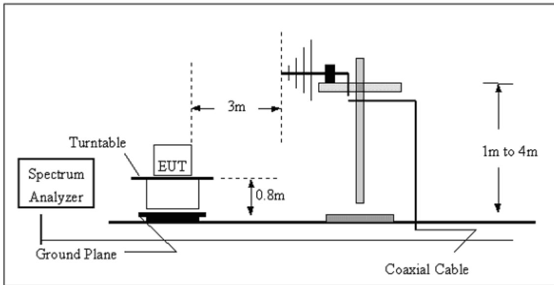
**(C) Radiated Emission Test-Up Frequency Above 1GHz**
