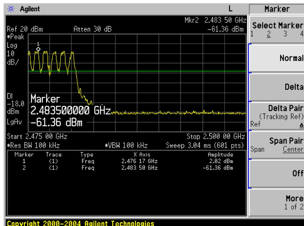
EDR mode ( $\pi/4$ -DQPSK): Band Edge-Left Side
