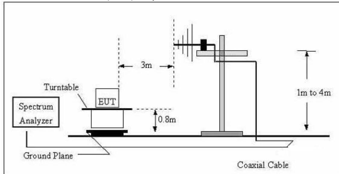
**(C) Radiated Emission Test-Up Frequency Above 1GHz**
