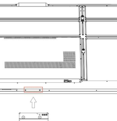
① Position the Sensor Box to the bottom of the Interactive Intelligent Panel in the direction of the arrow.
