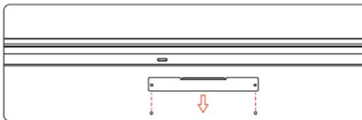
② Insert the wireless device fully into the tablet device along the direction of the arrow.
