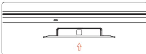
③ Secure the wireless device in place by tightening the removed screws to complete the installation.
