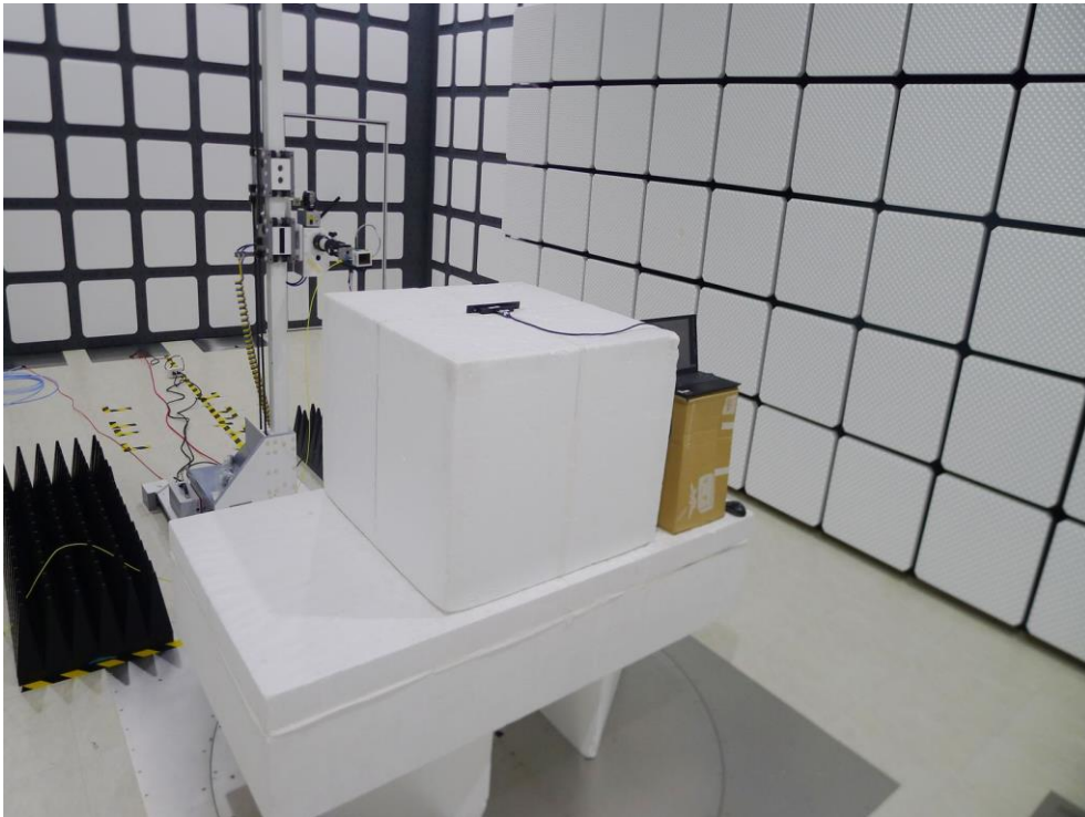
Description: Radiated Emission Test Setup for 9kHz~30MHz
