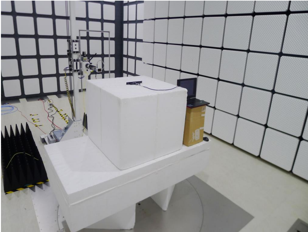
Description: Radiated Emission Test Setup for 9kHz~30MHz
