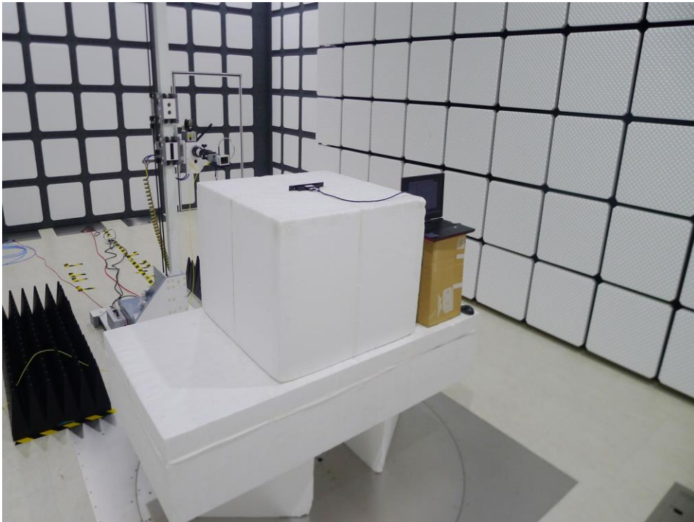
Description: Radiated Emission Test Setup for 9kHz~30MHz
