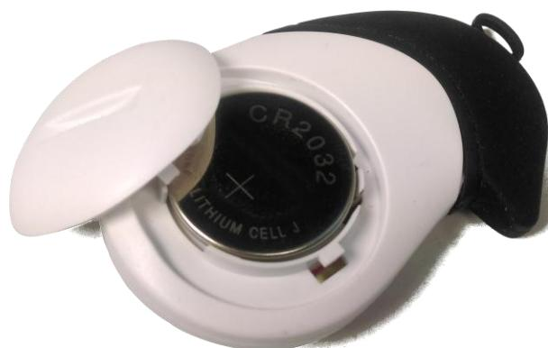
2. put the arrow which at battery cover to unlock mark, turn right battery cover until the arrow direct to lock mark.
