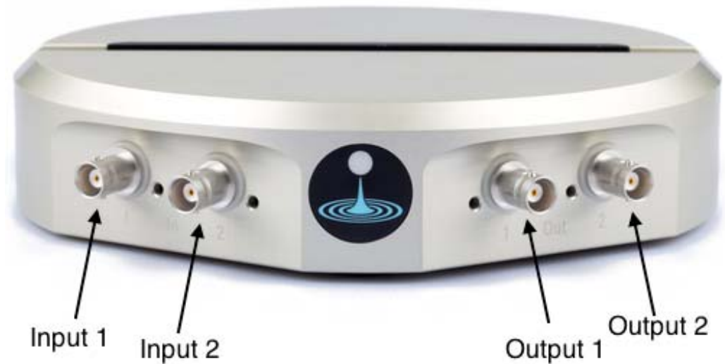
FIGURE 5: Front view of the Liquid Instruments Moku. The front interface shows two 200MHz inputs and two 200MHz outputs. The logo/button in between the inputs and outputs lights up with different colors to provide a state identifier.
