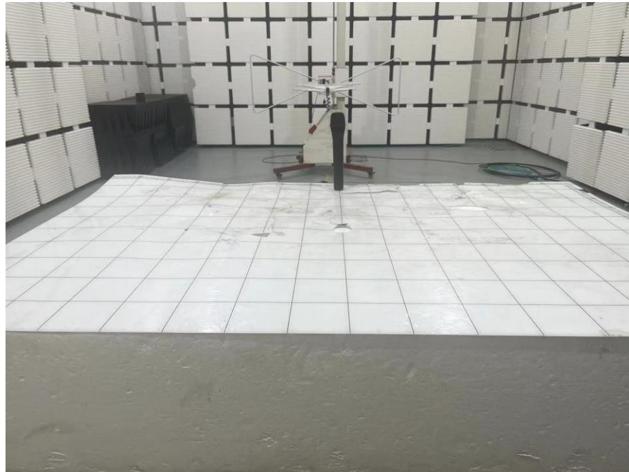
**Set-up for Radiated Emission (RE), Above 1GHz**
