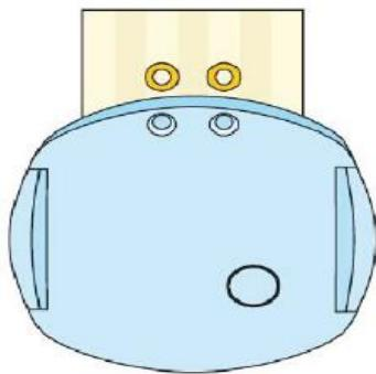
9: Press the host cover tightly to fix the sensor.
