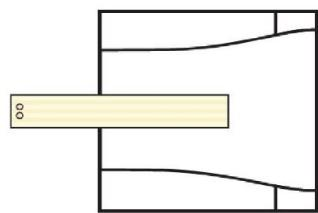
8: Correspond the location holes on the host with the holes on the sensor, three touch spots on the host is correspond with the metal plate on the sensor
