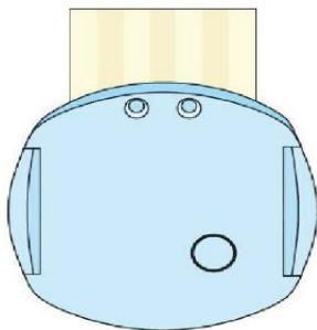
10: Press the switch in back side of host..If flash one time, that means the connection is successful. If flash three times, that means the connection is failed, and need to re-connect again.
