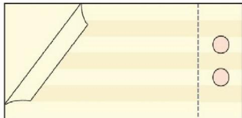
7; Stick the sensor in front of the diaper, and remain 35mm sensor with release paper outside of the diaper
